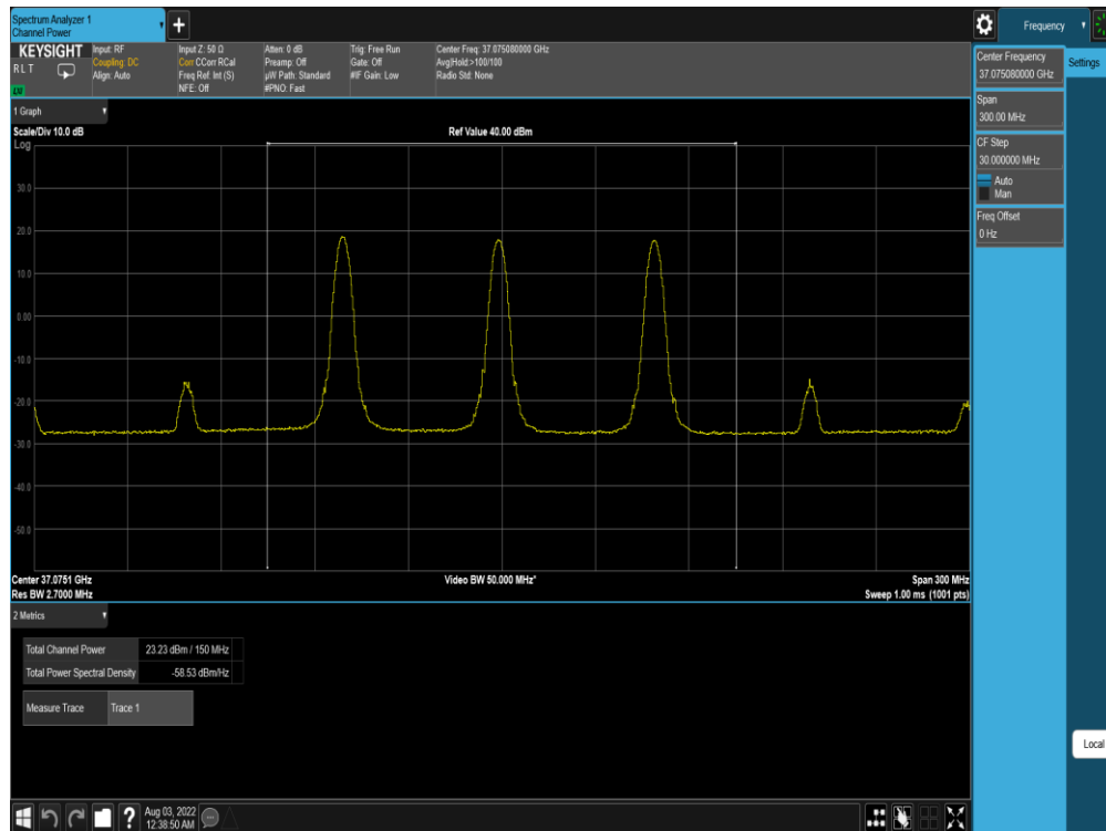
Plot 9-69. Ant M0 EIRP Plot (Band n260-50MHz-3CC SISO Dual Pol DFTs-OFDM – QPSK – Low Channel)
