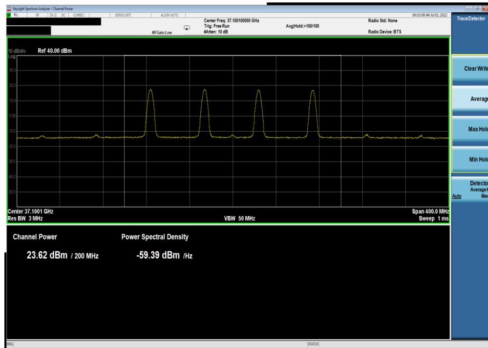
Plot 9-70. Ant M0 EIRP Plot (Band n260-50MHz-4CC SISO Dual Pol DFTs-OFDM – QPSK – Low Channel)
