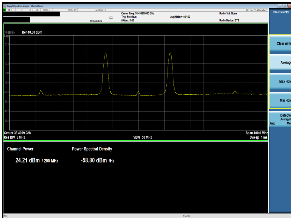
Plot 9-88. Ant M3 EIRP Plot (Band n260-100MHz-2CC SISO Dual Pol DFTs-OFDM – QPSK – Mid Channel)
