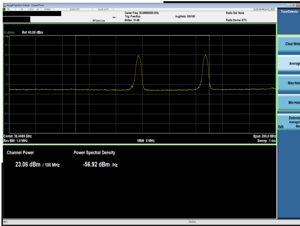
Plot 9-84. Ant M3 EIRP Plot (Band n260-50MHz-2CC MIMO CP-OFDM – QPSK – Mid Channel)
