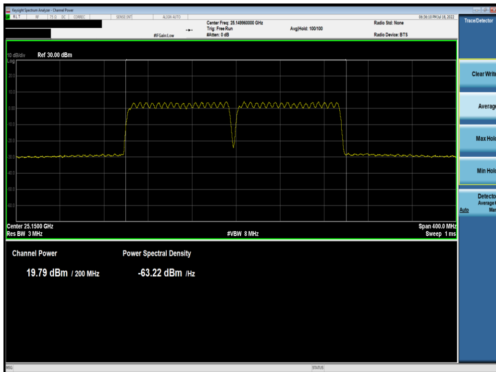
Plot 9-32. Ant M2 EIRP Plot (Band n258-R2-100MHz-2CC SISO Dual Pol DFTs-OFDM – 16QAM – High Channel)
