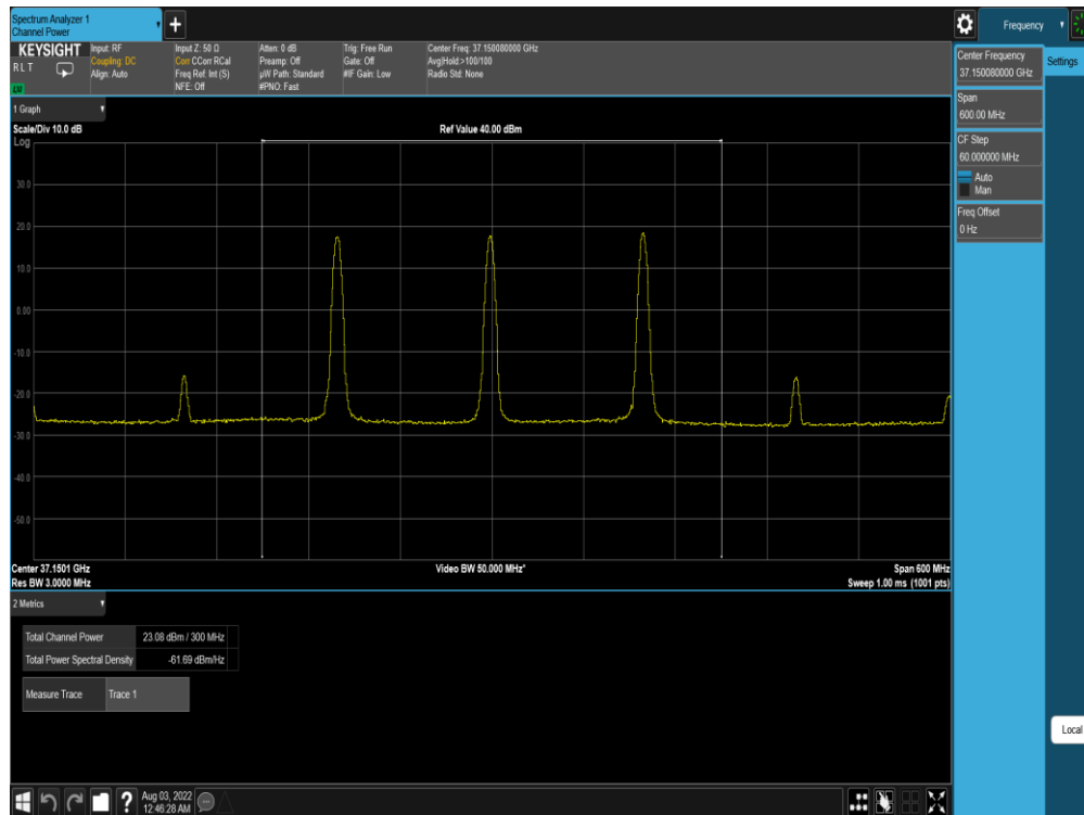
Plot 9-73. Ant M0 EIRP Plot (Band n260-100MHz-3CC SISO Dual Pol DFTs-OFDM – \pi/2 BPSK – Low Channel)
