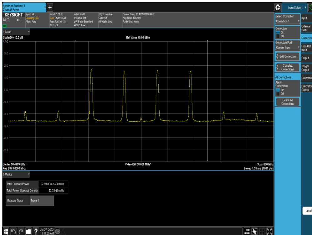
Plot 9-82. Ant M2 EIRP Plot (Band n260-100MHz-4CC MIMO CP-OFDM – 16QAM – Mid Channel)
