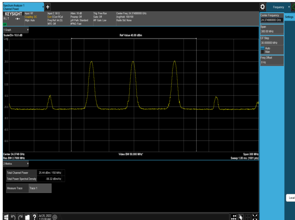
Plot 9-3. Ant M0 EIRP Plot (Band n258-R1-50MHz-3CC SISO Dual Pol DFTs-OFDM – QPSK – High Channel)
