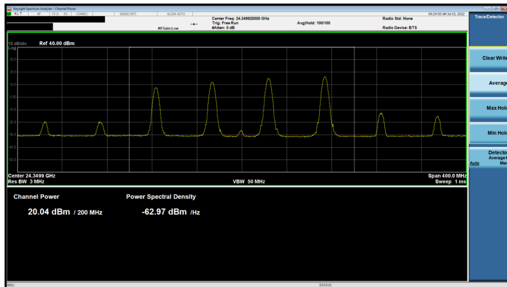
Plot 9-10. Ant M2 EIRP Plot (Band n258-R1-50MHz-4CC SISO Dual Pol DFTs-OFDM – \pi/2 BPSK – Mid Channel)
