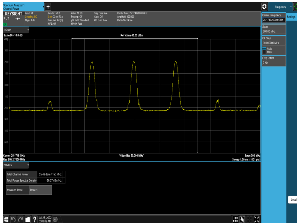
Plot 9-21. Ant M0 EIRP Plot (Band n258-R2-50MHz-3CC SISO Dual Pol DFTs-OFDM – QPSK – High Channel)
