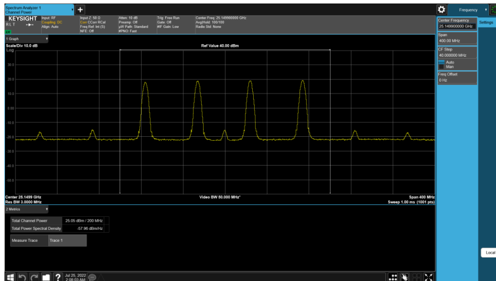
Plot 9-22. Ant M0 EIRP Plot (Band n258-R2-50MHz-4CC SISO Dual Pol DFTs-OFDM – \pi/2 -BPSK – High Channel)
