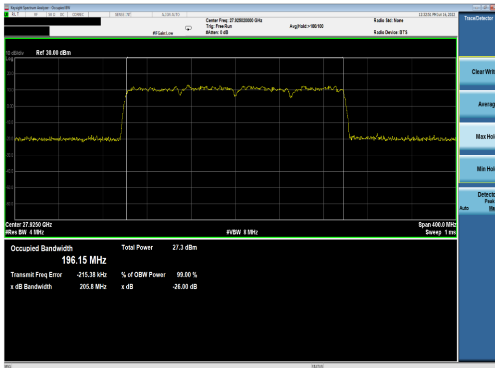
Plot 7-252. Ant M0 OBW (Band n261-50MHz-4CC SISO Dual Pol DFTs-OFDM – 64QAM – Mid Channel)
