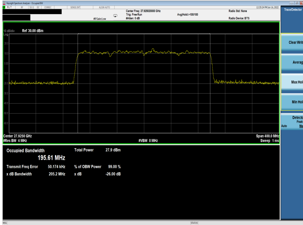
Plot 7-249. Ant M0 OBW (Band n261-50MHz-4CC SISO Dual Pol DFTs-OFDM – \pi/2 BPSK – Mid Channel)
