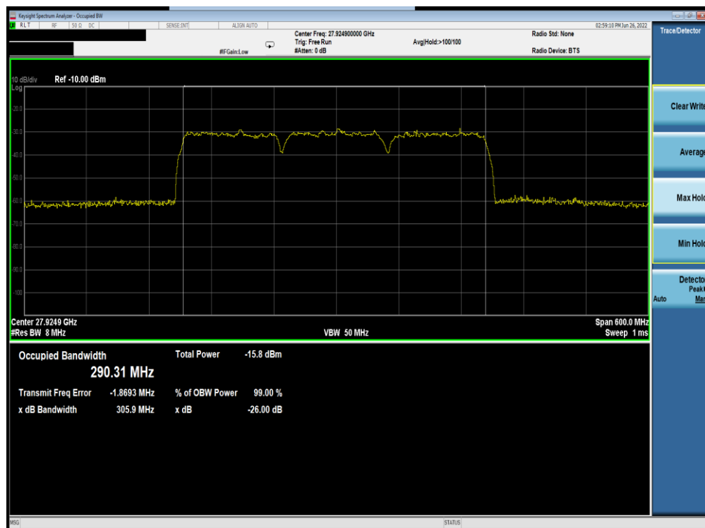
Plot 7-292. Ant M0 OBW (Band n261-100MHz-3CC SISO Dual Pol DFTs-OFDM – QPSK – Mid Channel)
