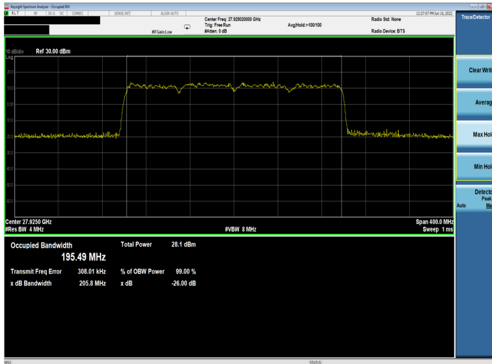
Plot 7-250. Ant M0 OBW (Band n261-50MHz-4CC SISO Dual Pol DFTs-OFDM – QPSK – Mid Channel)
