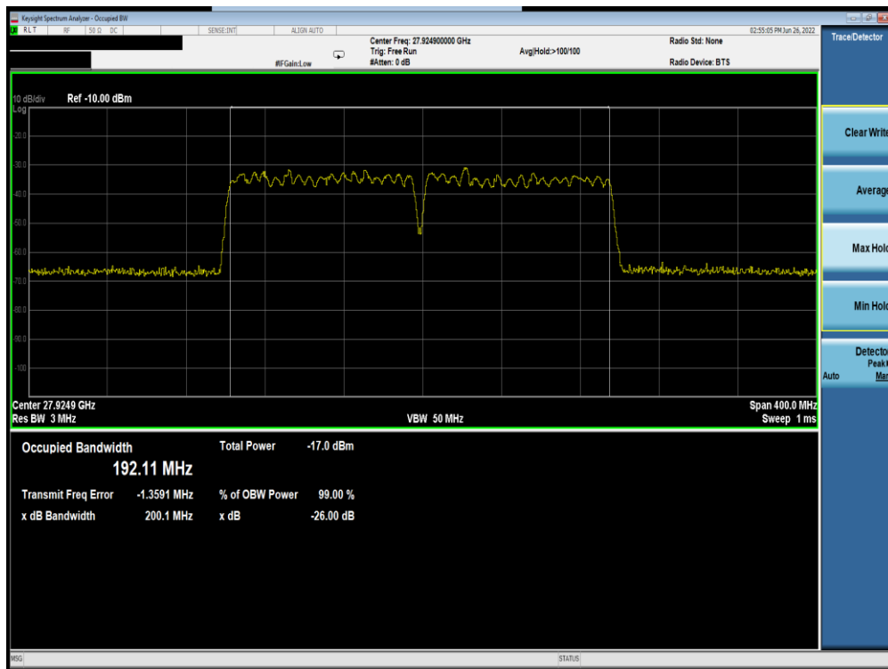
Plot 7-280. Ant M0 OBW (Band n261-100MHz-2CC SISO Dual Pol DFTs-OFDM – 64QAM – Mid Channel)
