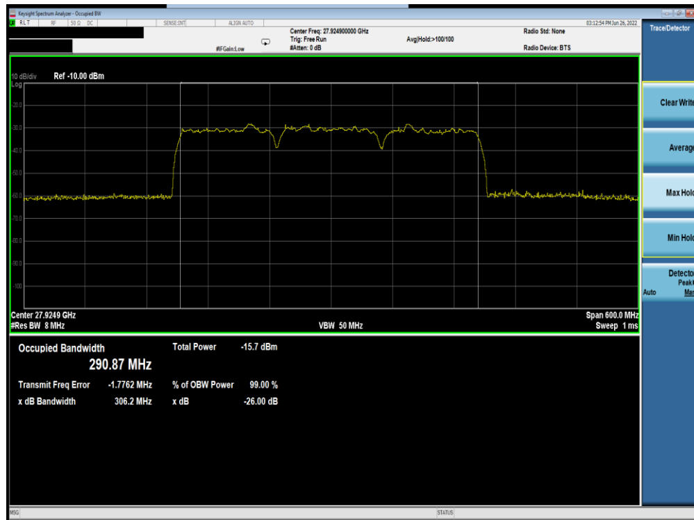
Plot 7-291. Ant M0 OBW (Band n261-100MHz-3CC SISO Dual Pol DFTs-OFDM – \pi/2 BPSK – Mid Channel)
