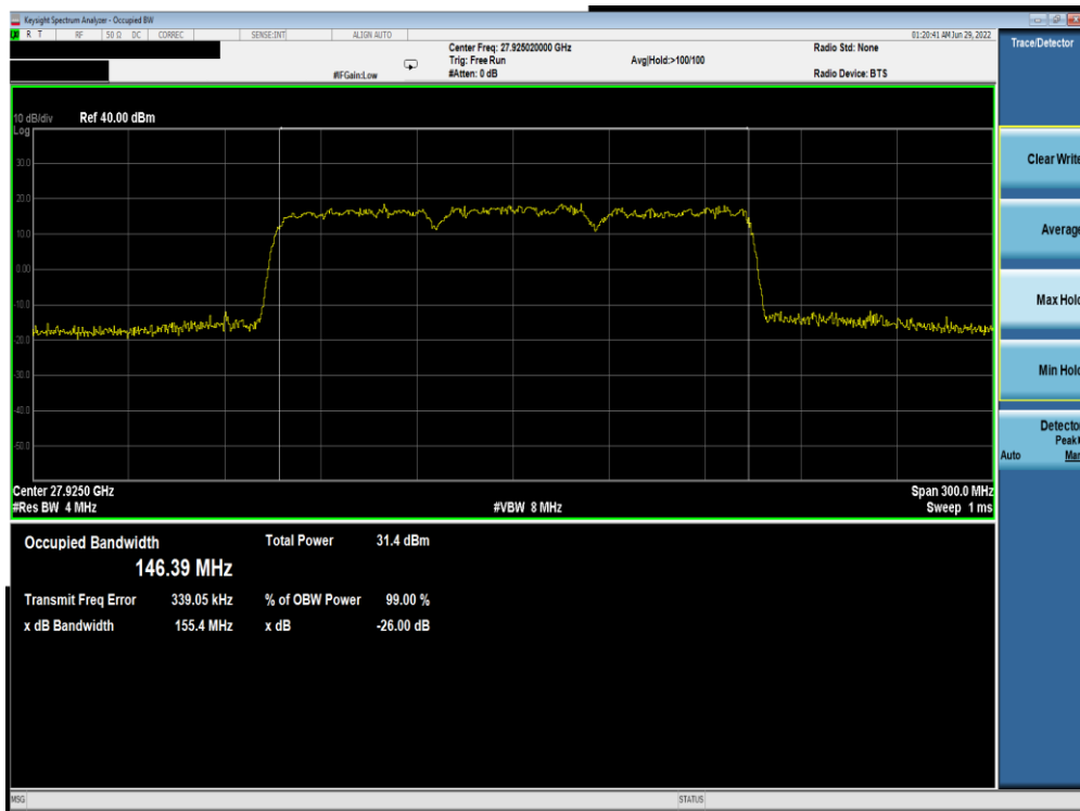
Plot 7-232. Ant M0 OBW (Band n261-50MHz-3CC MIMO CP-OFDM – QPSK – Mid Channel)
