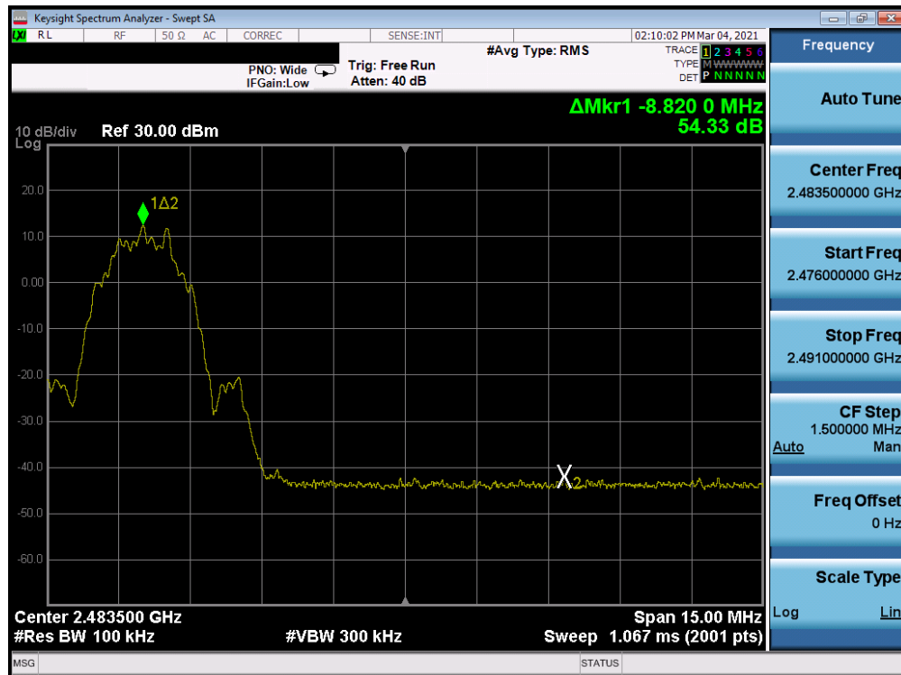
Plot 7-68. Band Edge Plot Antenna 7 (Bluetooth (LE), 2Mbps, ePA – Ch. 38)
