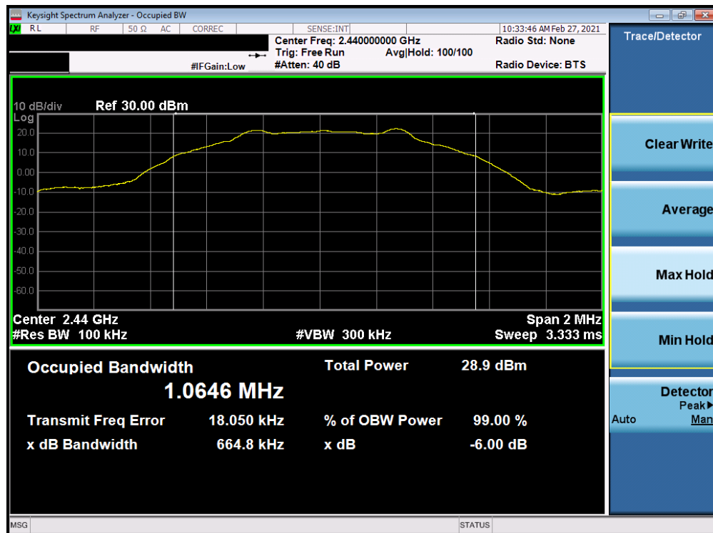
Plot 7-8. 6dB BW & 99% OBW Plot Antenna 7 (Bluetooth (LE), 1Mbps, ePA – Ch. 19)
