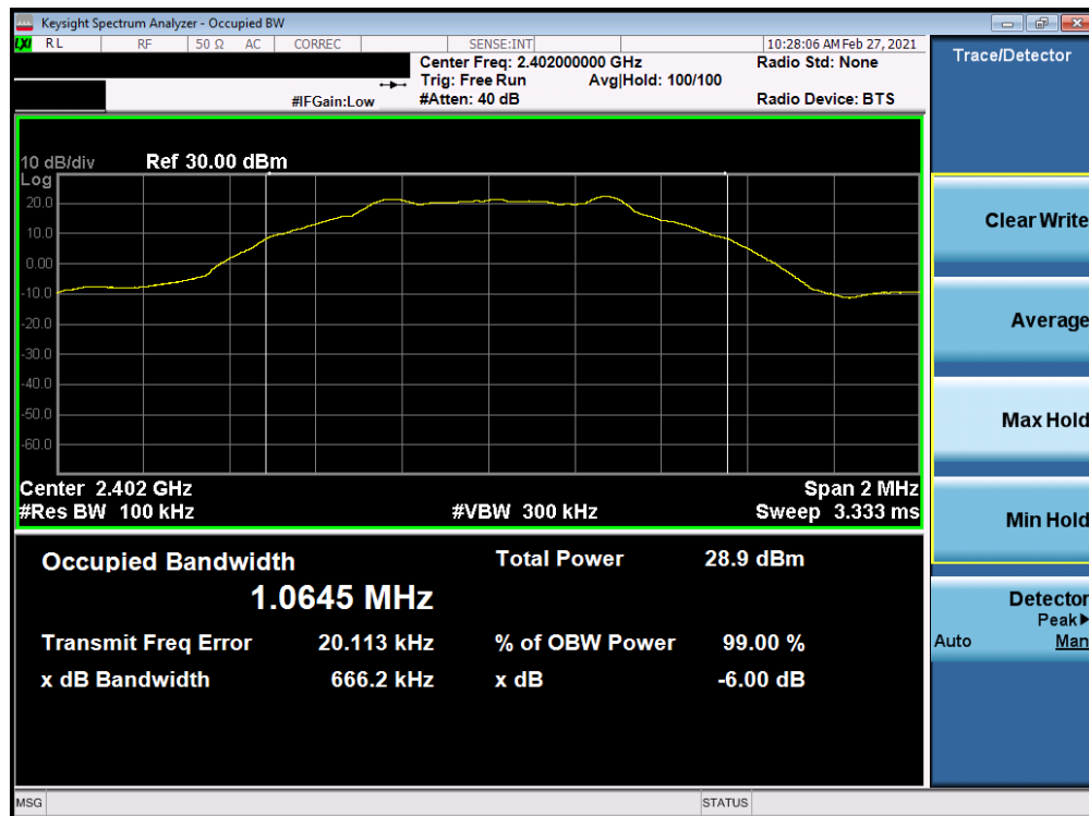
Plot 7-7. 6dB BW & 99% OBW Plot Antenna 7 (Bluetooth (LE), 1Mbps, ePA – Ch. 0)
