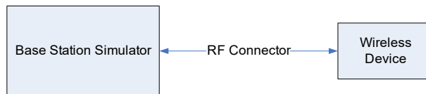
Figure 8-2 Power Measurement Setup
