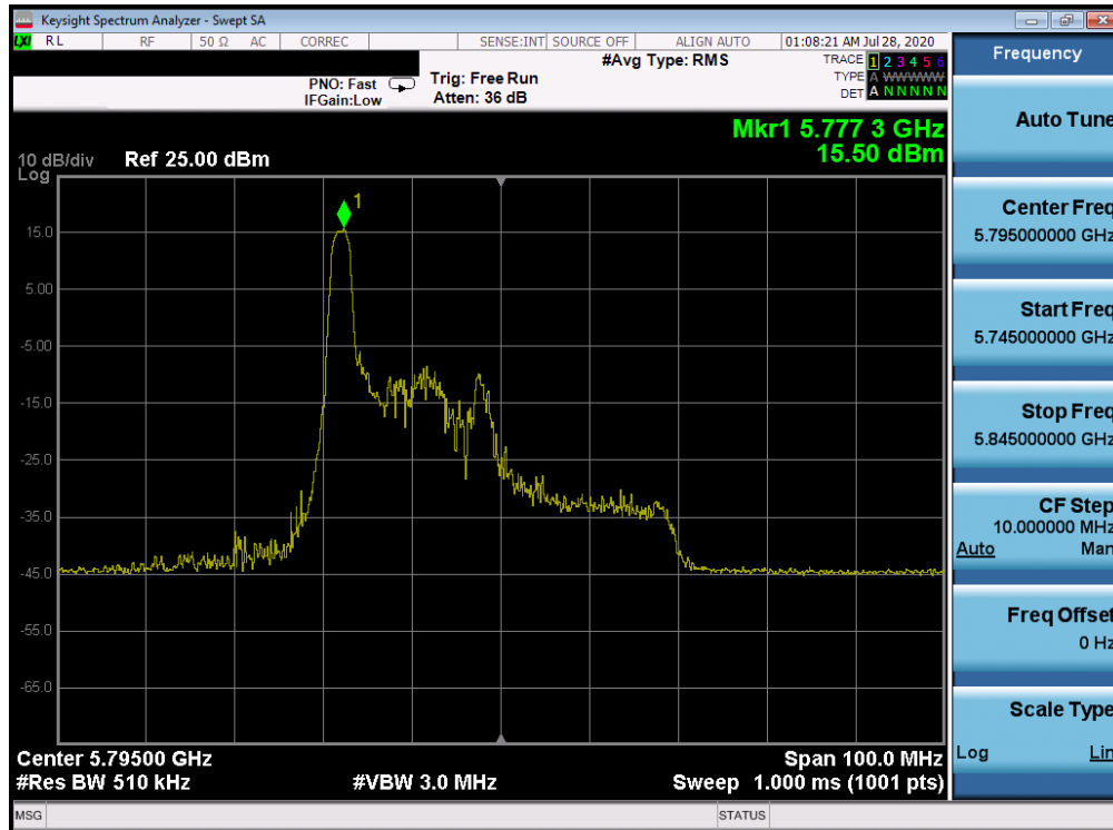
Plot 7-655. Power Spectral Density Plot CDD ANT WF8 (40MHz BW 802.11ax Index 0 – RU26 (UNII Band 3) – Ch. 159)
