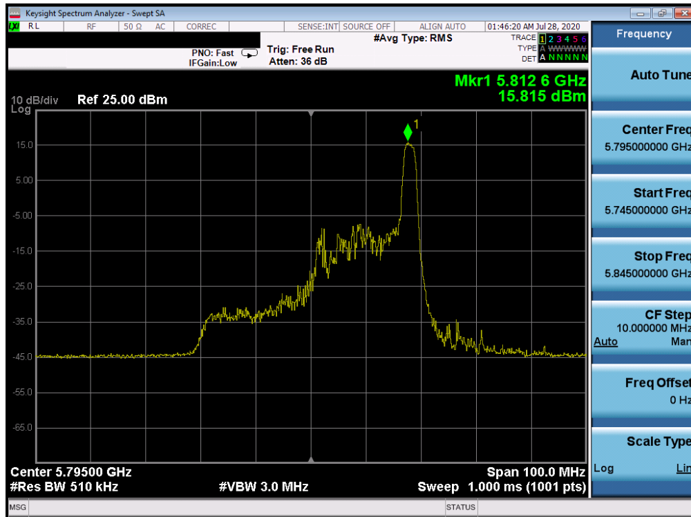
Plot 7-659. Power Spectral Density Plot CDD ANT WF8 (40MHz BW 802.11ax Index 17 – RU26 (UNII Band 3) – Ch. 159)
