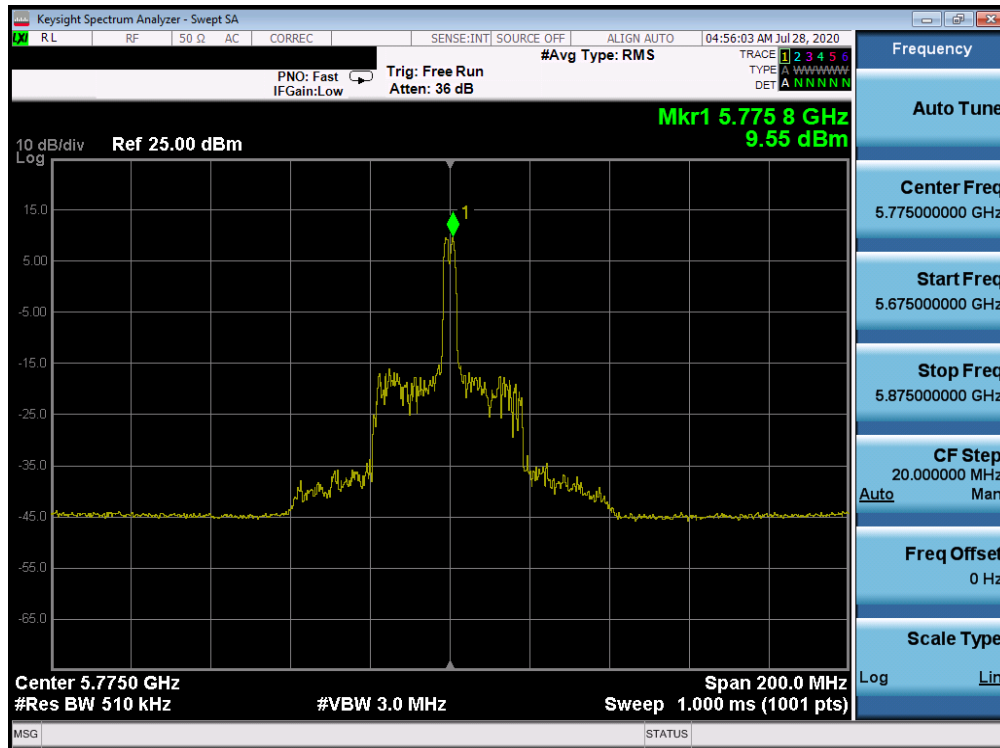
Plot 7-667. Power Spectral Density Plot CDD ANT WF8 (80MHz BW 802.11ax Index 18 – RU26 (UNII Band 3) – Ch. 155)
