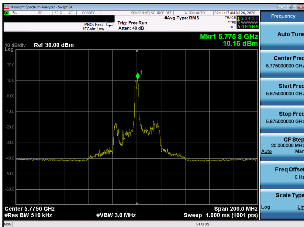
Plot 7-438. Power Spectral Density Plot ANT WF7a (80MHz BW 802.11ax Index 18 – RU26 (UNII Band 3) – Ch. 155)
