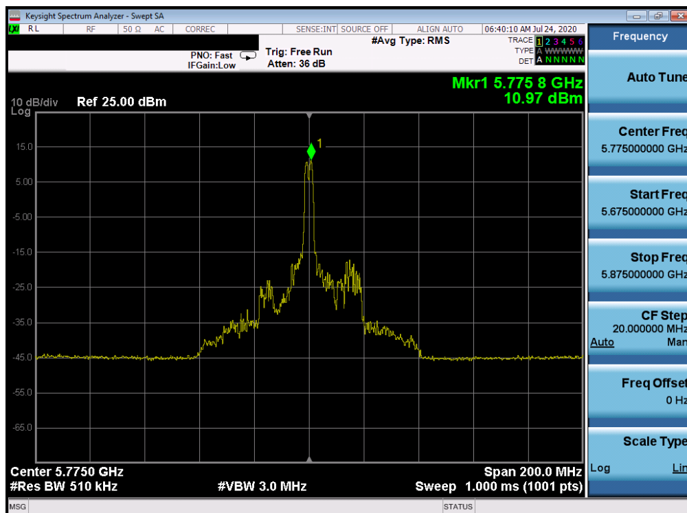
Plot 7-310. Power Spectral Density Plot ANT WF8 (80MHz BW 802.11ax Index 18 – RU26 (UNII Band 3) – Ch. 155)
