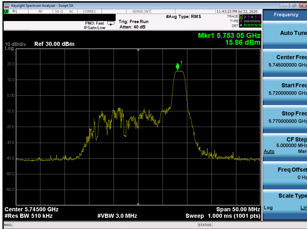
Plot 7-291. Power Spectral Density Plot ANT WF8 (20MHz BW 802.11ax Index 8 – RU26 (UNII Band 3) – Ch. 149)
