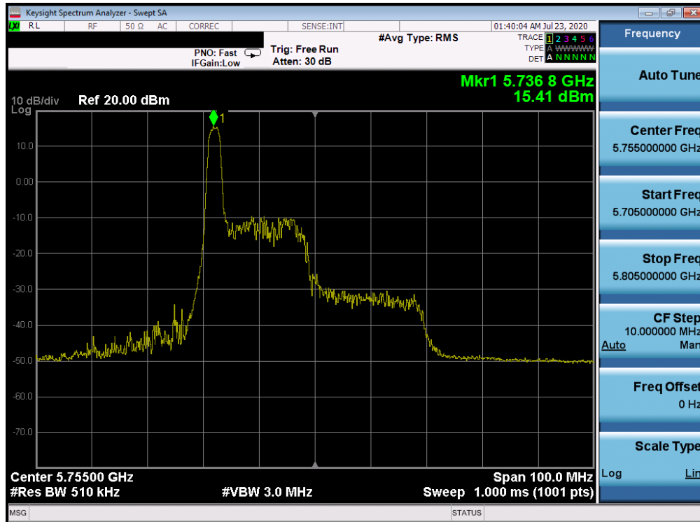
Plot 7-301. Power Spectral Density Plot ANT WF8 (40MHz BW 802.11ax Index 0 – RU26 (UNII Band 3) – Ch. 151)
