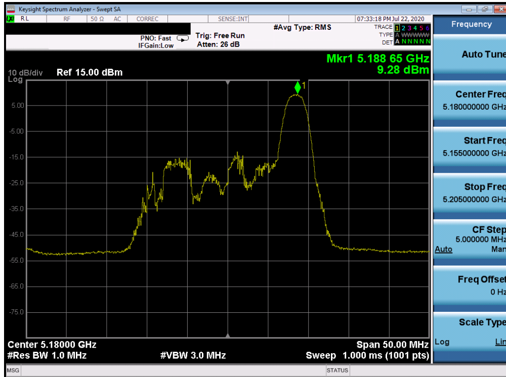
Plot 7-211. Power Spectral Density Plot ANT WF8 (20MHz BW 802.11ax Index 8 – RU26 (UNII Band 1) – Ch. 36)
