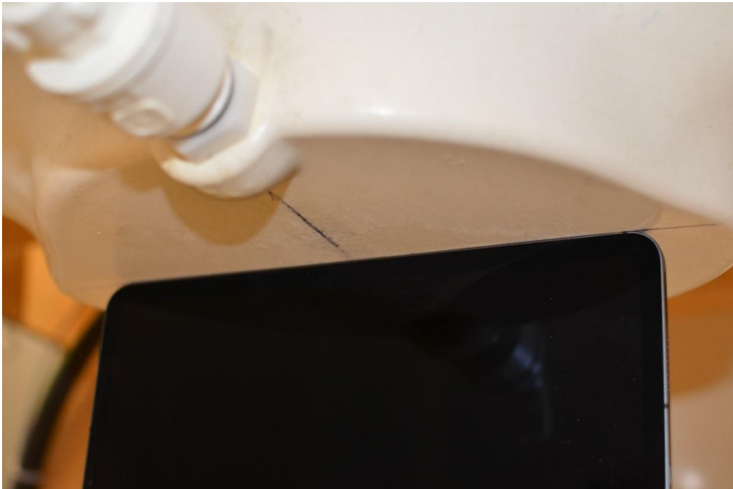
SAR Test Setup Photo 6: Right Edge at 0.0 cm
