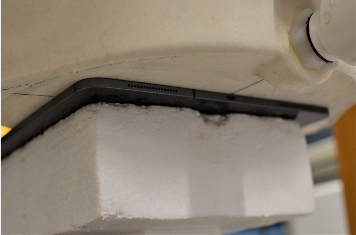
SAR Test Setup Photo 3: Back Side at 0.0 cm – Ant 1/2A/2B
