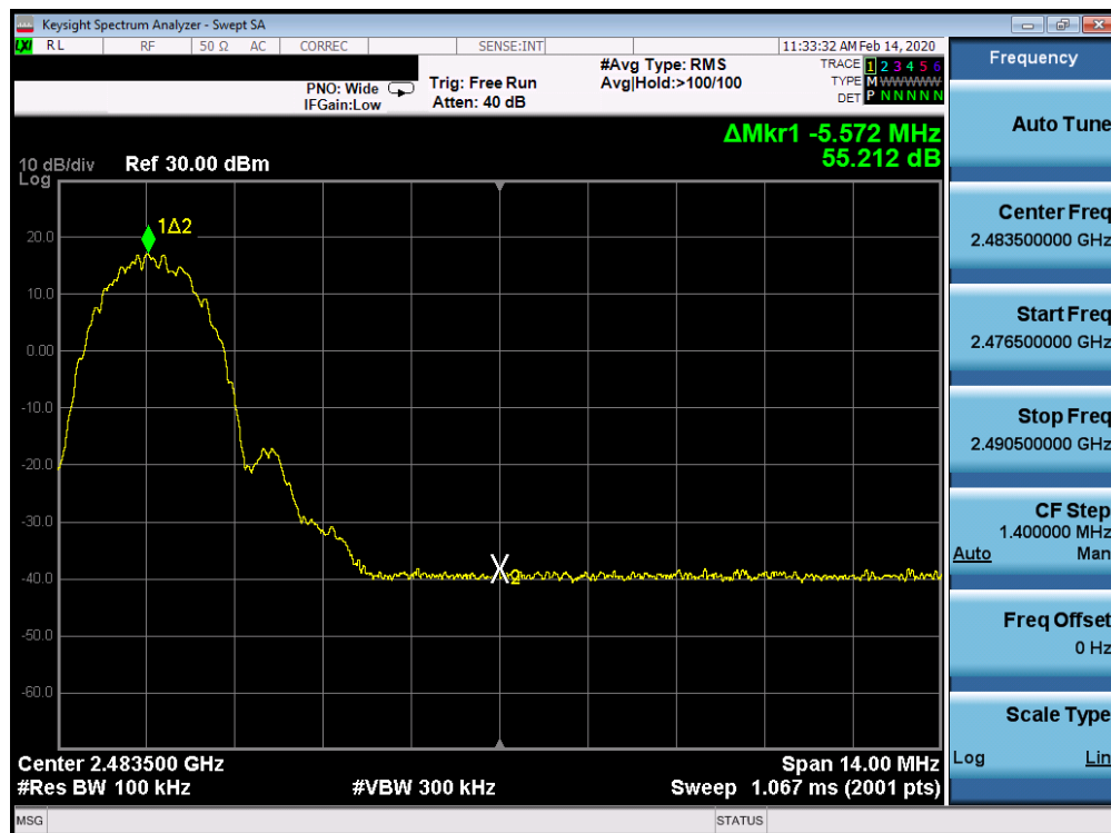
Plot 7-68. Band Edge Plot Ant 2a (Bluetooth (LE), 2Mbps ePA – Ch. 38)
