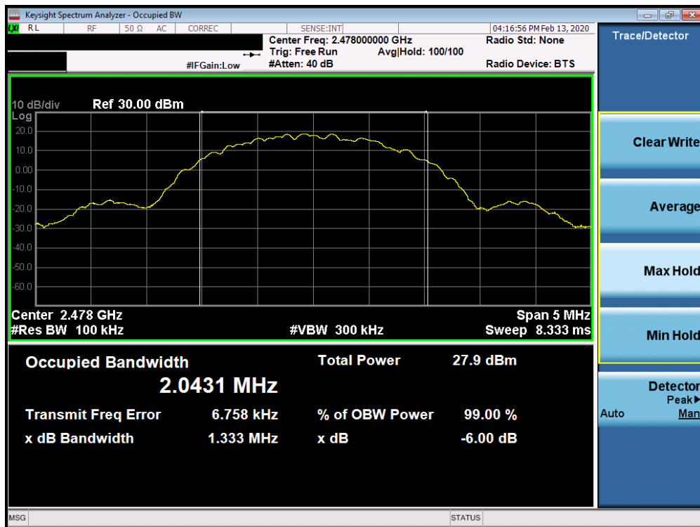
Plot 7-6. 6dB Bandwidth Plot Ant 4a (Bluetooth (LE), 2Mbps, ePA – Ch. 38)
