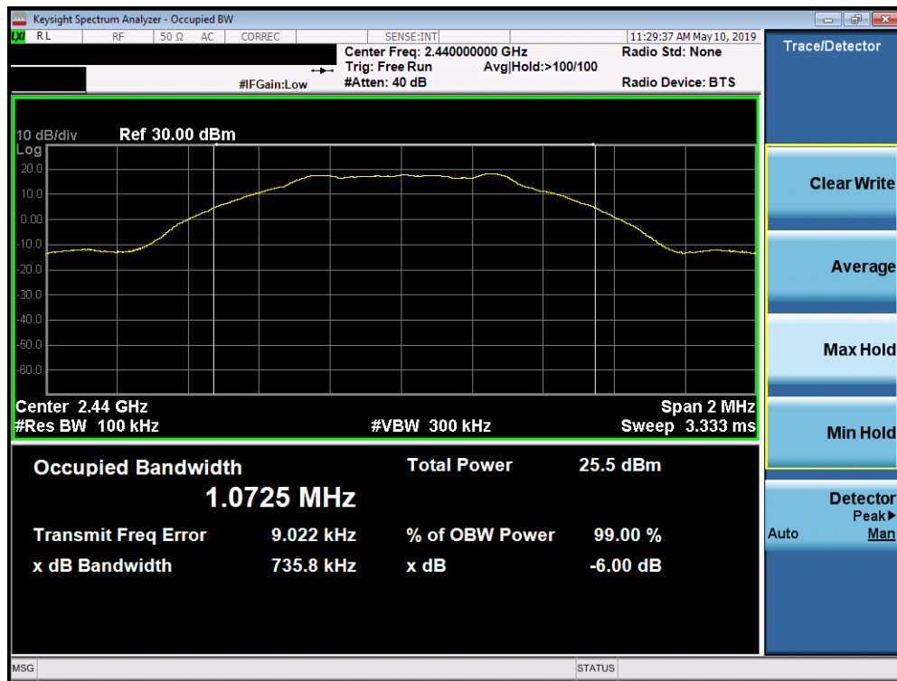
Plot 7-2. 6dB Bandwidth Plot (Bluetooth (LE), ePA – Ch. 19)
