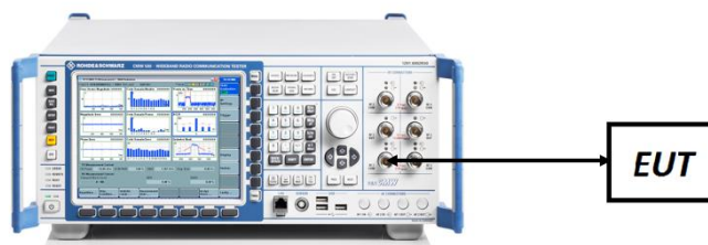
Figure 7-7. ERP/EIRP Measurement Setup
