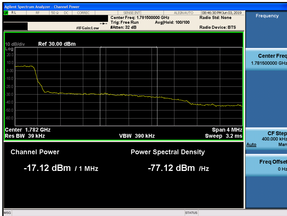
Plot 7-208. Upper Extended Band Edge Plot (Band 66 - 3.0MHz QPSK - Full RB Configuration)
