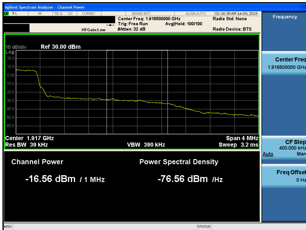
Plot 7-256. Upper Extended Band Edge Plot (Band 25 - 3.0MHz QPSK - Full RB Configuration)
