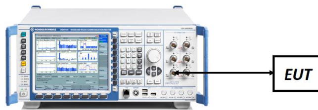
Figure 7-5. ERP/EIRP Measurement Setup
