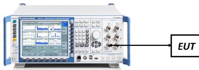
Figure 7-5. ERP/EIRP Measurement Setup
