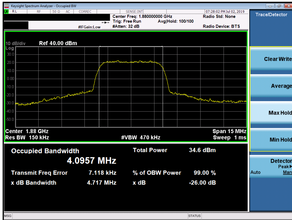
Plot 7-7. Occupied Bandwidth Plot (PCS WCDMA Mode)
