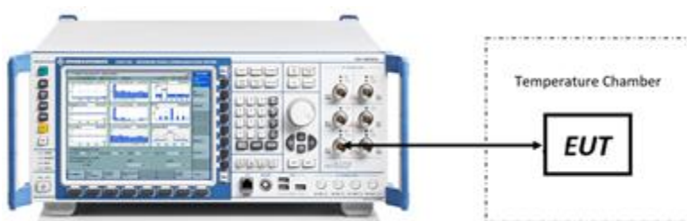
Figure 7-8. Test Instrument & Measurement Setup
