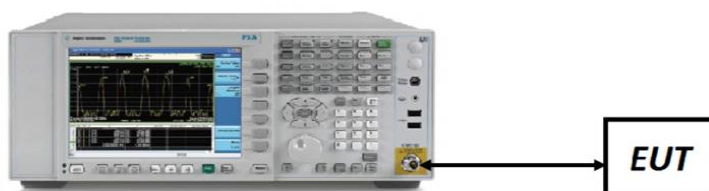
Figure 7-6. Test Instrument & Measurement Setup
