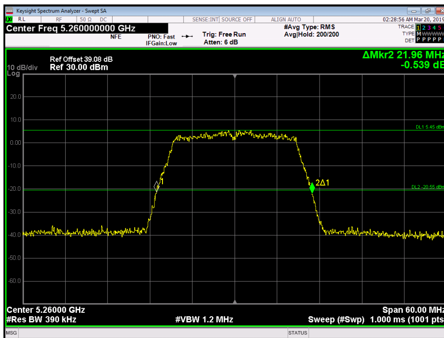
Figure 119 - 5260 MHz - 26 dB Emission Bandwidth
