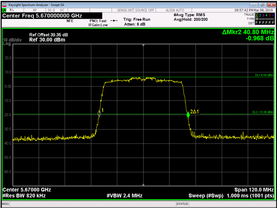
Figure 211 - 5670 MHz - 26 dB Emission Bandwidth
