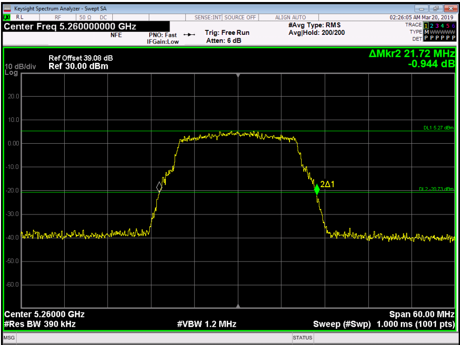
Figure 113 - 5260 MHz - 26 dB Emission Bandwidth
