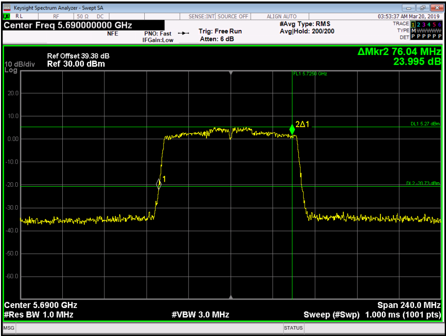
Figure 249 - 5690 MHz - 26 dB Emission Bandwidth
