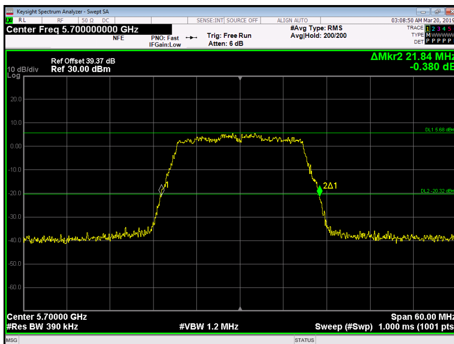
Figure 187 - 5700 MHz - 26 dB Emission Bandwidth
