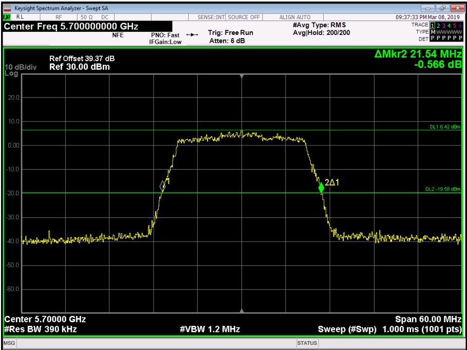
Figure 195 - 5700 MHz - 26 dB Emission Bandwidth
