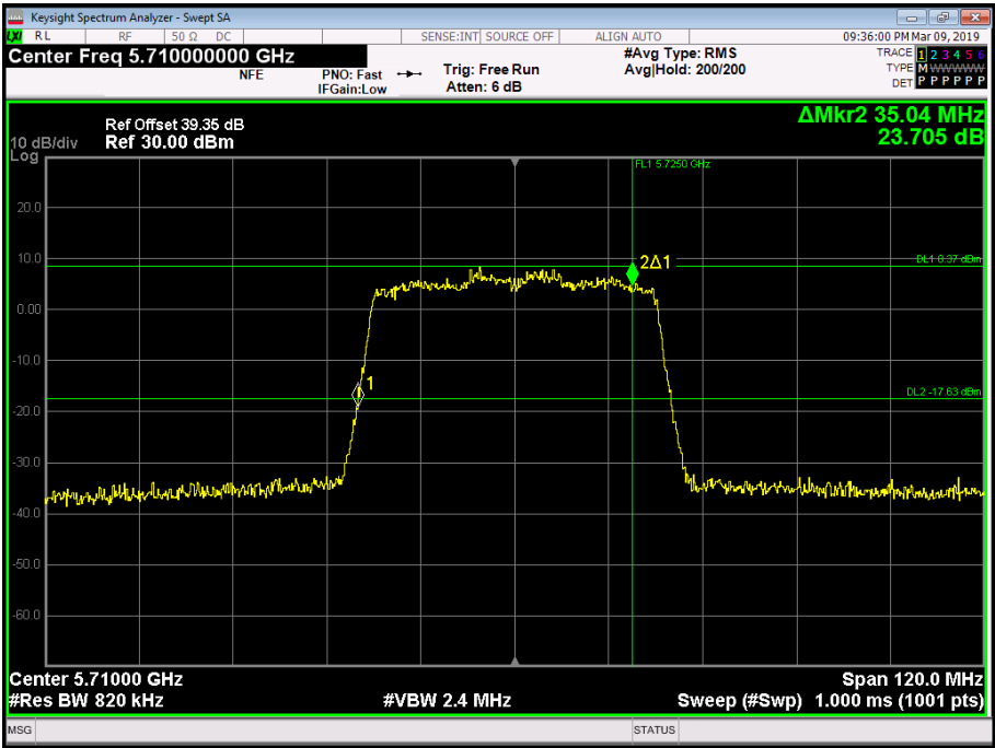
Figure 221 - 5710 MHz - 26 dB Emission Bandwidth
