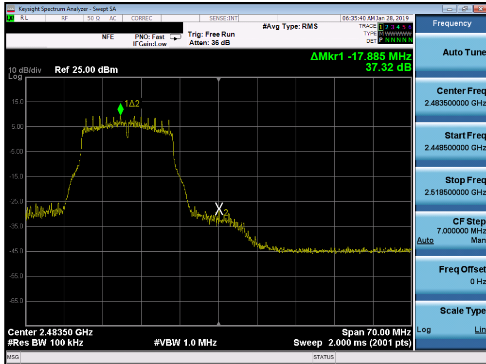
Plot 7-67. Band Edge Plot SISO CORE 1 (802.11g – Ch. 12)
