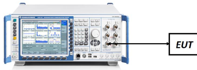
Figure 7-5. ERP Measurement Setu
