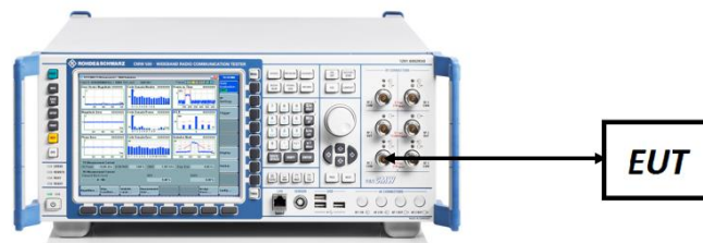
Figure 7-4. Conducted Power Measurement Setup
