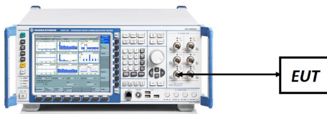
Figure 7-5. ERP/EIRP Measurement Setup
