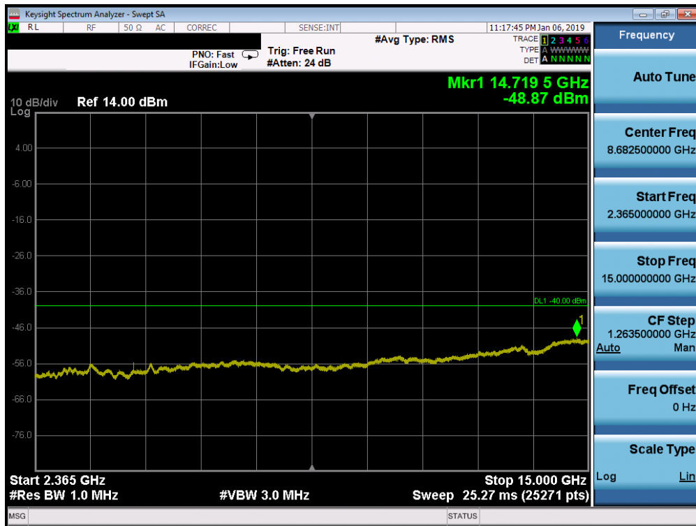
Plot 7-164. Conducted Spurious Plot (Band 30 - 5.0MHz QPSK - RB Size 1, RB Offset 0 - Low Channel)
