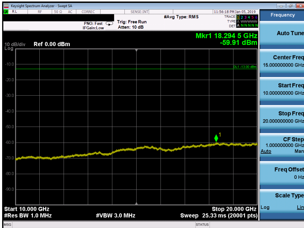
Plot 7-150. Conducted Spurious Plot (Band 66/4 - 20.0MHz QPSK - RB Size 1, RB Offset 0 - Mid Channel)
