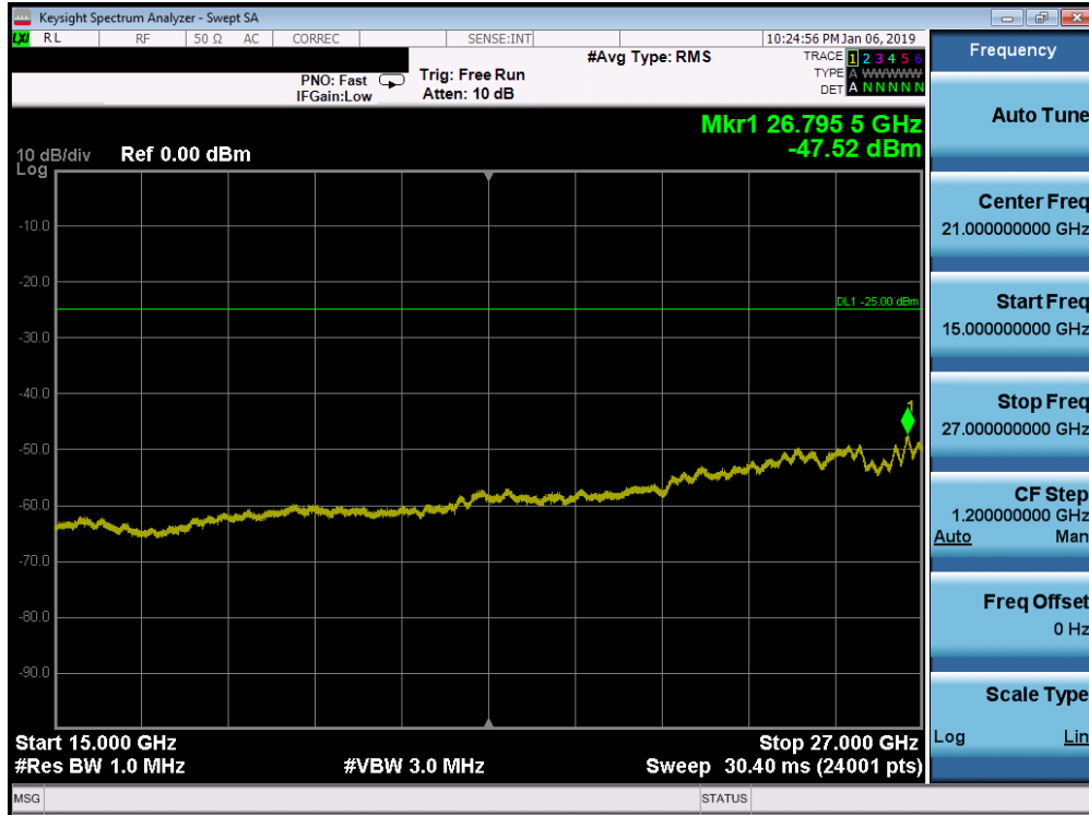
Plot 7-180. Conducted Spurious Plot (Band 7 - 20.0MHz QPSK - RB Size 1, RB Offset 0 - High Channel)
