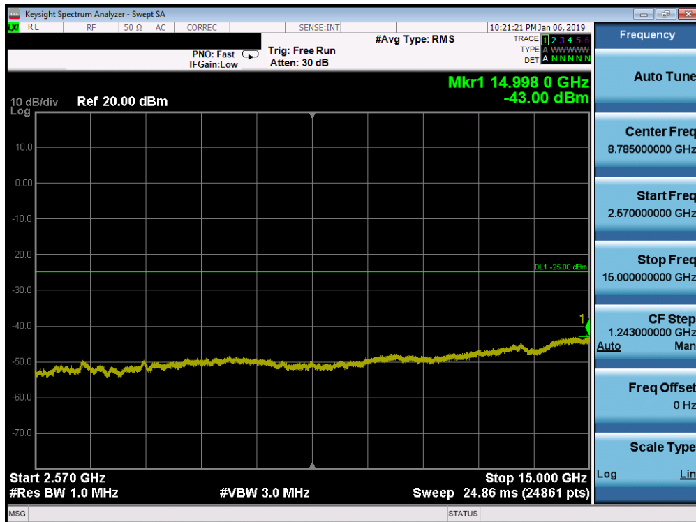
Plot 7-173. Conducted Spurious Plot (Band 7 - 20.0MHz QPSK - RB Size 1, RB Offset 0 - Low Channel)
