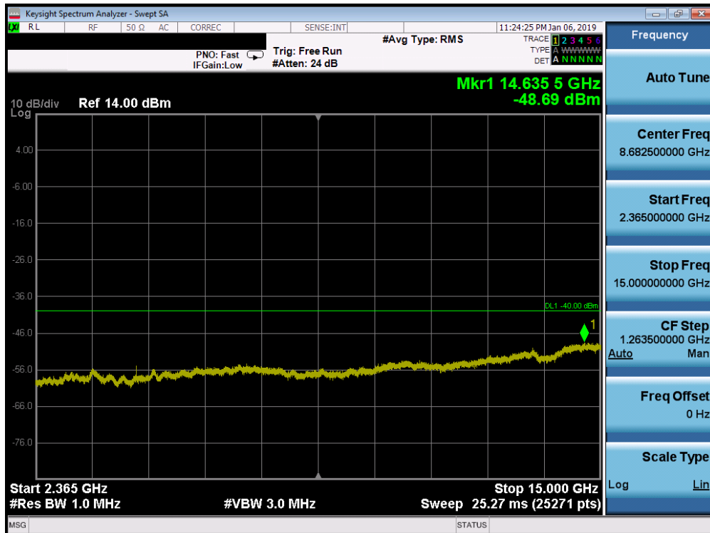
Plot 7-170. Conducted Spurious Plot (Band 30 - 5.0MHz QPSK - RB Size 1, RB Offset 0 - High Channel)
