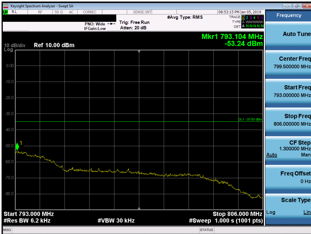
Plot 7-213. Higher Emission Mask Edge Plot (Band 13 - 5.0MHz QPSK - Full RB Configuration)
