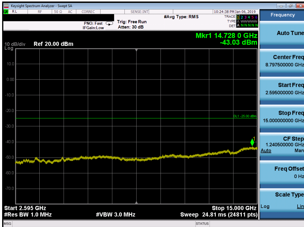
Plot 7-179. Conducted Spurious Plot (Band 7 - 20.0MHz QPSK - RB Size 1, RB Offset 0 - High Channel)
