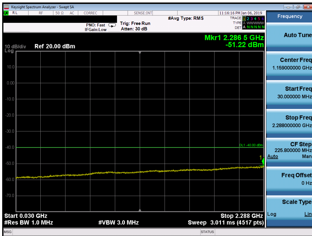
Plot 7-166. Conducted Spurious Plot (Band 30 - 5.0MHz QPSK - RB Size 1, RB Offset 0 - Mid Channel)
