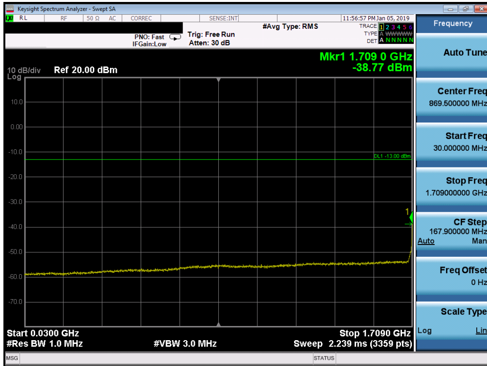
Plot 7-145. Conducted Spurious Plot (Band 66/4 - 20.0MHz QPSK - RB Size 1, RB Offset 0 - Low Channel)
