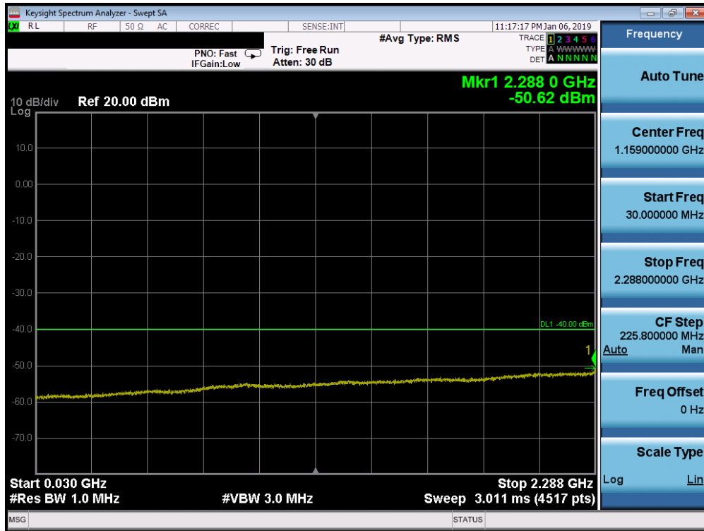
Plot 7-163. Conducted Spurious Plot (Band 30 - 5.0MHz QPSK - RB Size 1, RB Offset 0 - Low Channel)
