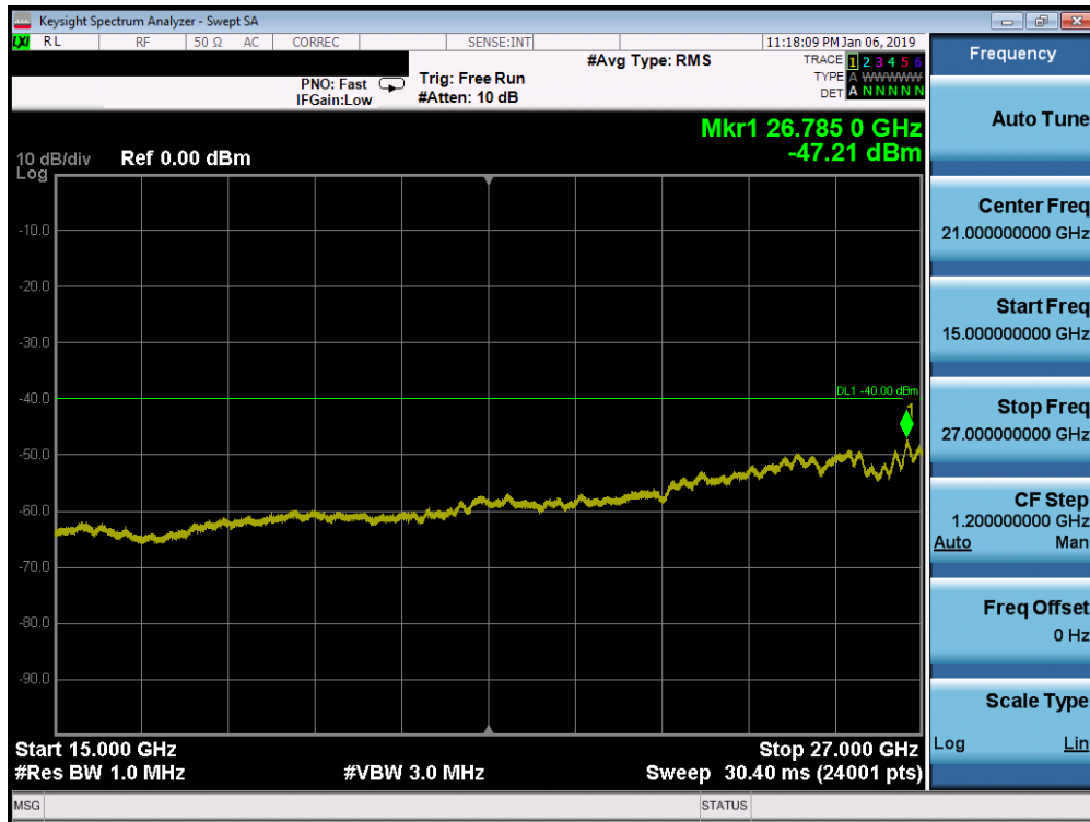
Plot 7-165. Conducted Spurious Plot (Band 30 - 5.0MHz QPSK - RB Size 1, RB Offset 0 - Low Channel)
