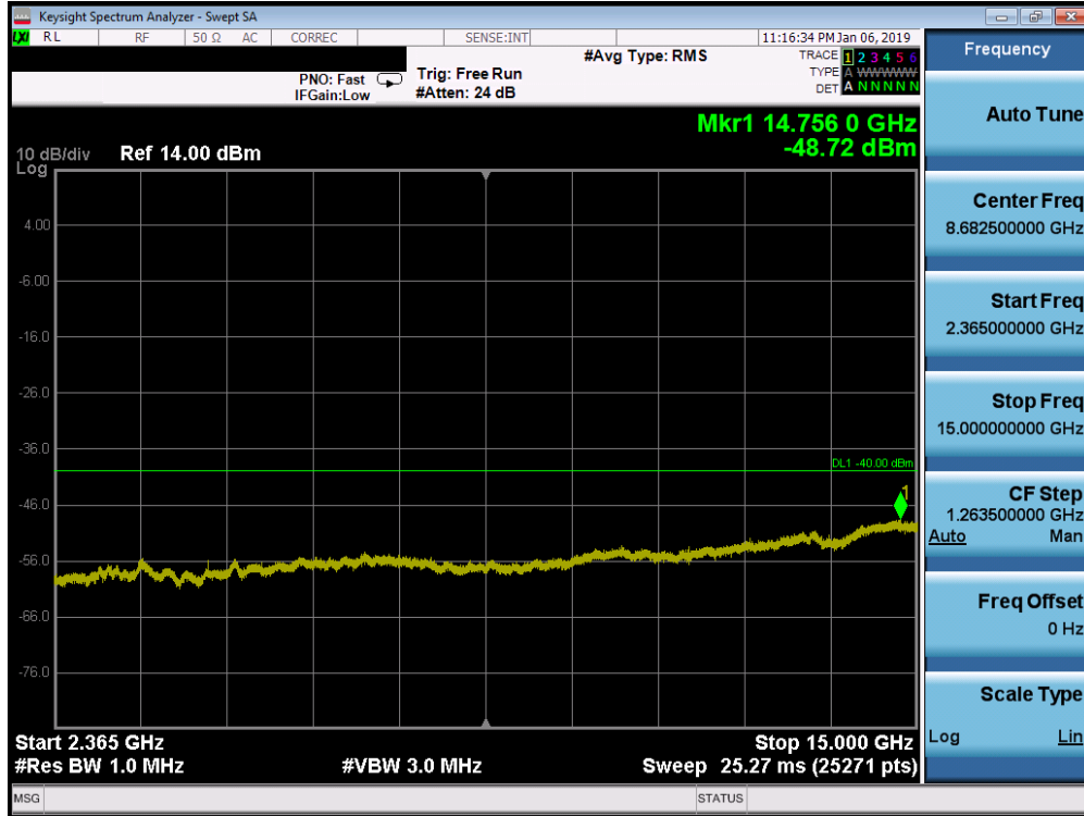
Plot 7-167. Conducted Spurious Plot (Band 30 - 5.0MHz QPSK - RB Size 1, RB Offset 0 - Mid Channel)
