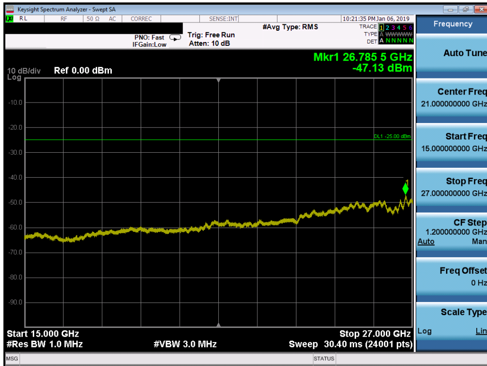
Plot 7-174. Conducted Spurious Plot (Band 7 - 20.0MHz QPSK - RB Size 1, RB Offset 0 - Low Channel)
