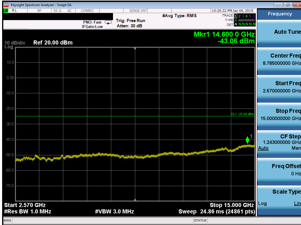
Plot 7-176. Conducted Spurious Plot (Band 7 - 20.0MHz QPSK - RB Size 1, RB Offset 0 - Mid Channel)
