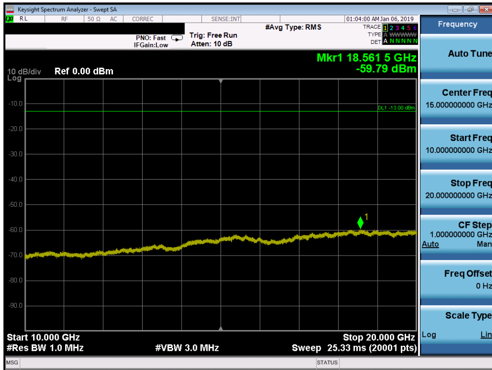
Plot 7-156. Conducted Spurious Plot (Band 25/2 - 20.0MHz QPSK - RB Size 1, RB Offset 0 - Low Channel)
