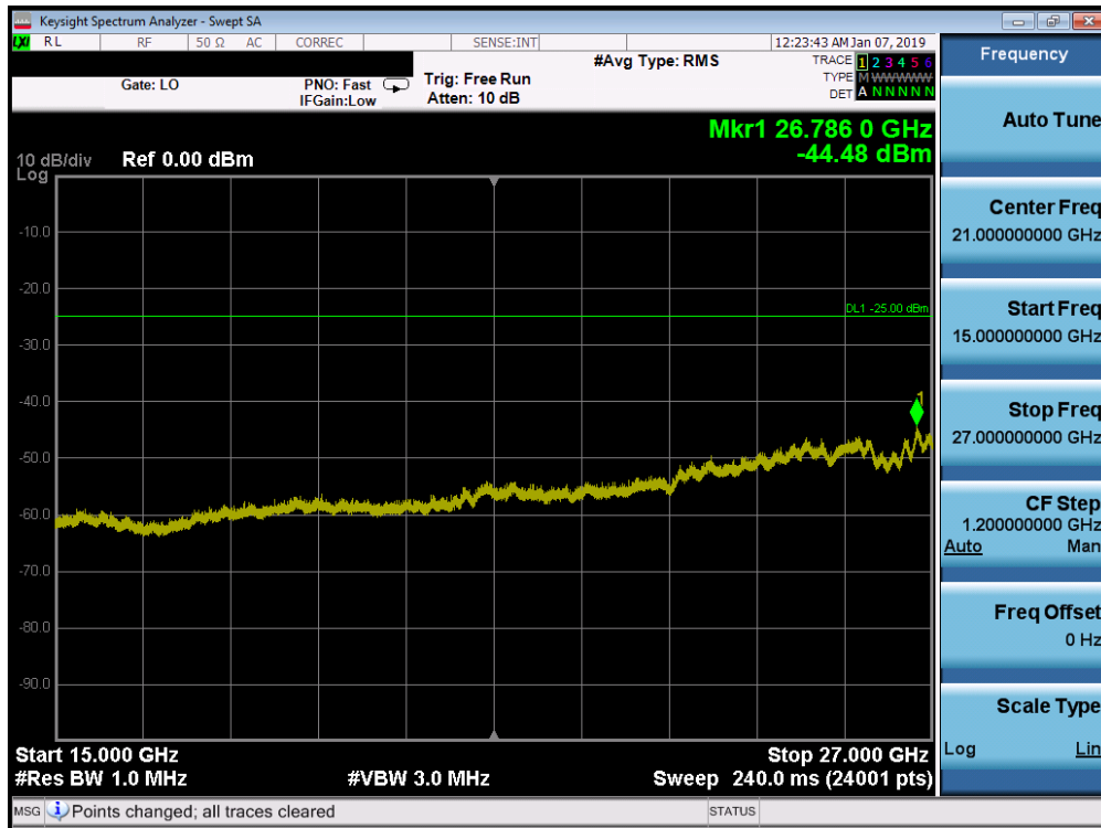
Plot 7-183. Conducted Spurious Plot (Band 41 - 20.0MHz QPSK - RB Size 1, RB Offset 0 - Low Channel)
