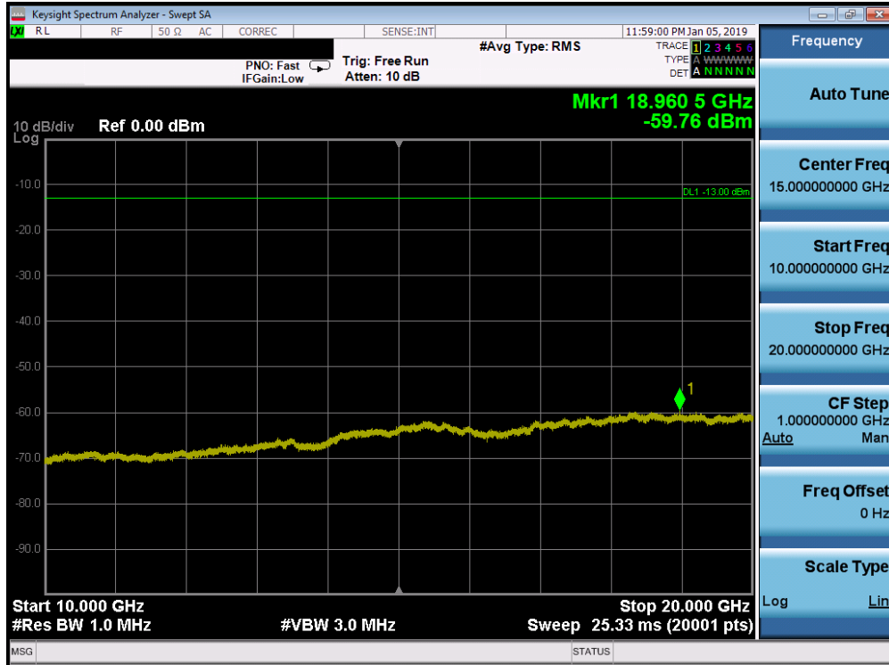
Plot 7-153. Conducted Spurious Plot (Band 66/4 - 20.0MHz QPSK - RB Size 1, RB Offset 0 - High Channel)
