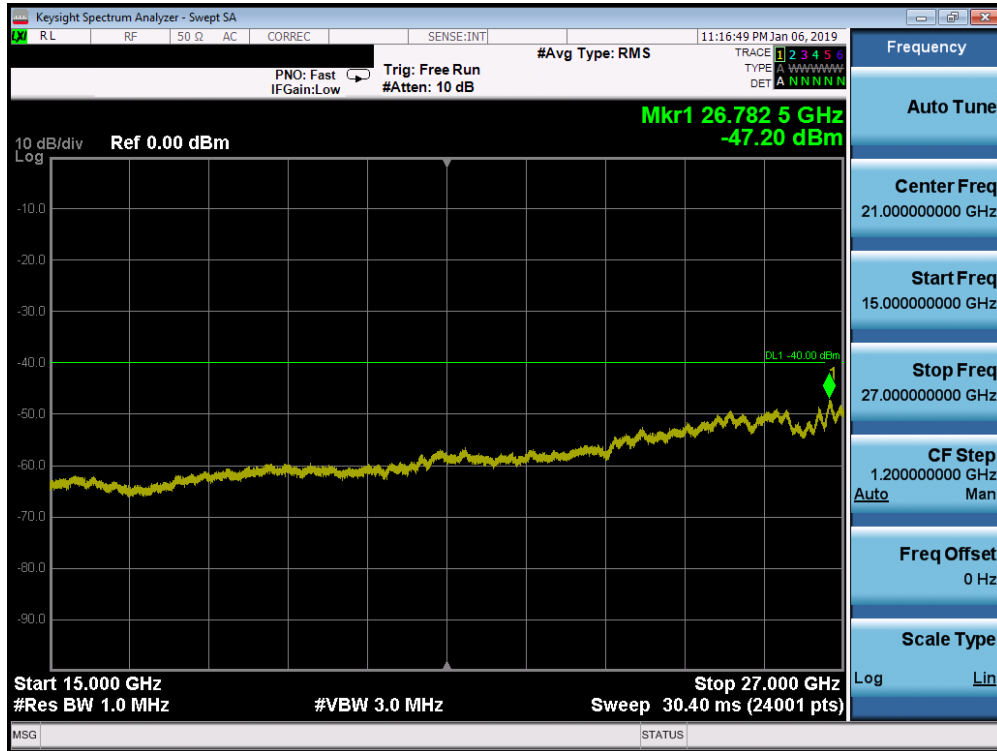
Plot 7-168. Conducted Spurious Plot (Band 30 - 5.0MHz QPSK - RB Size 1, RB Offset 0 - Mid Channel)
