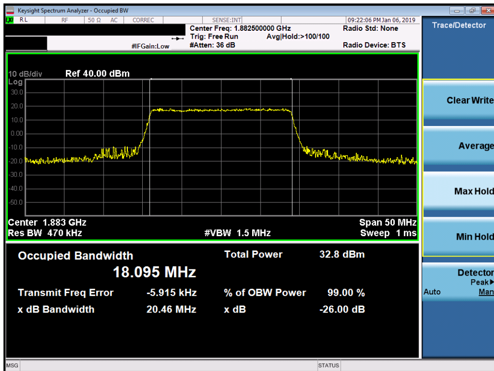
Plot 7-78. Occupied Bandwidth Plot (Band 25/2 - 20.0MHz 64-QAM - Full RB Configuration)
