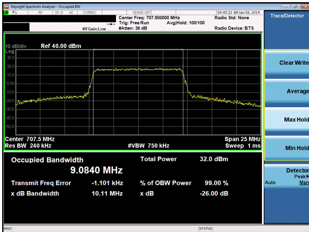
Plot 7-24. Occupied Bandwidth Plot (Band 12/17 - 10.0MHz 64-QAM - Full RB Configuration)
