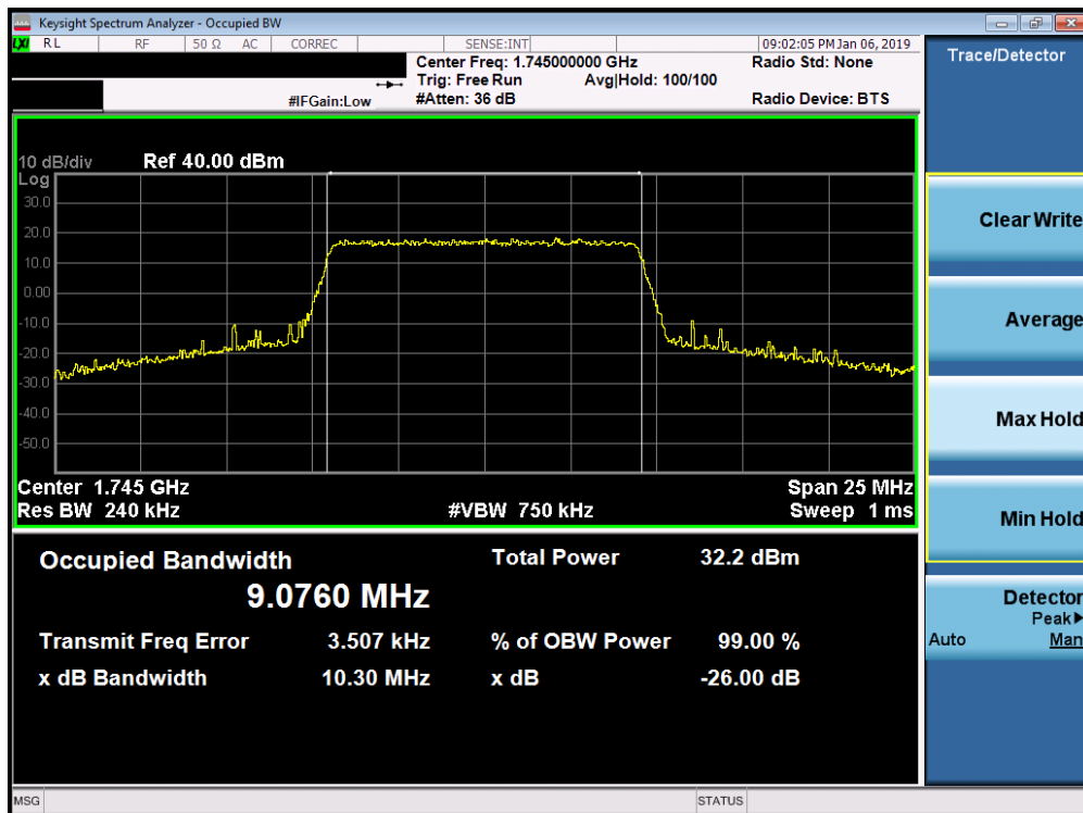
Plot 7-54. Occupied Bandwidth Plot (Band 66/4 - 10.0MHz 64-QAM - Full RB Configuration)
