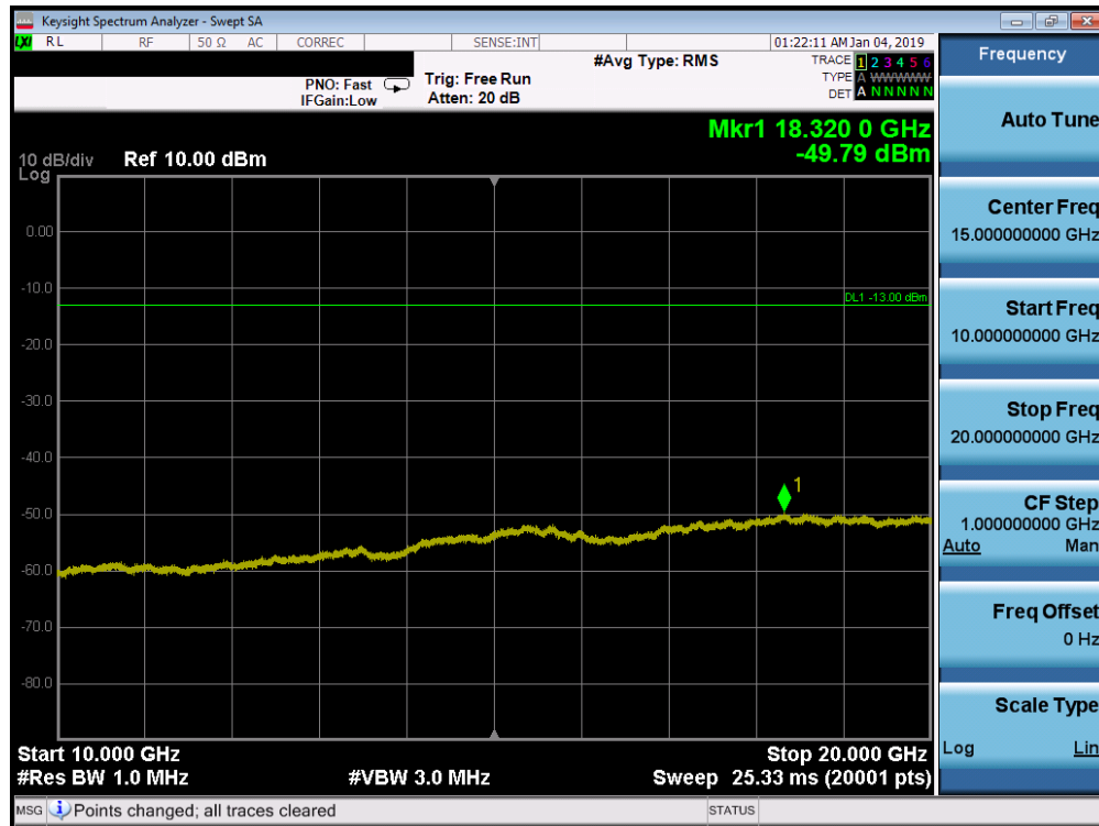
Plot 7-52. Conducted Spurious Plot (PCS WCDMA Mode - High Channel)
