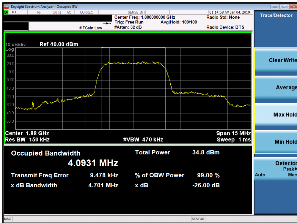
Plot 7-7. Occupied Bandwidth Plot (PCS WCDMA Mode)
