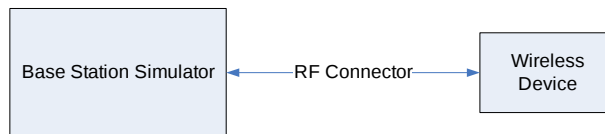
Figure 8-1 Power Measurement Setup
