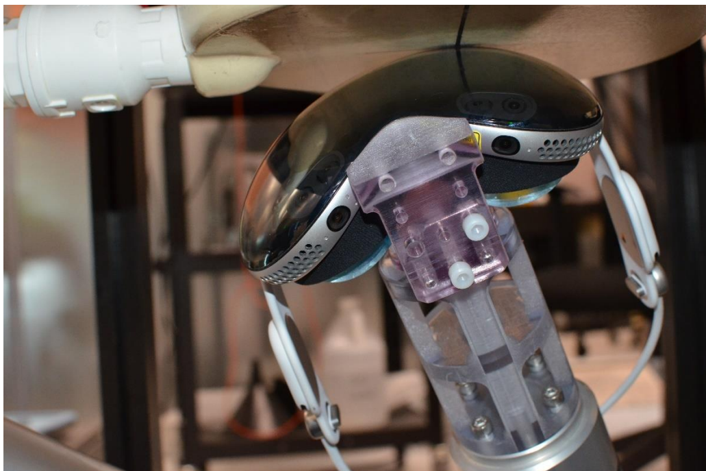
SAR Test Setup Photo 29: Antenna 2 Point 11 Extremity SAR at 0.0 cm
