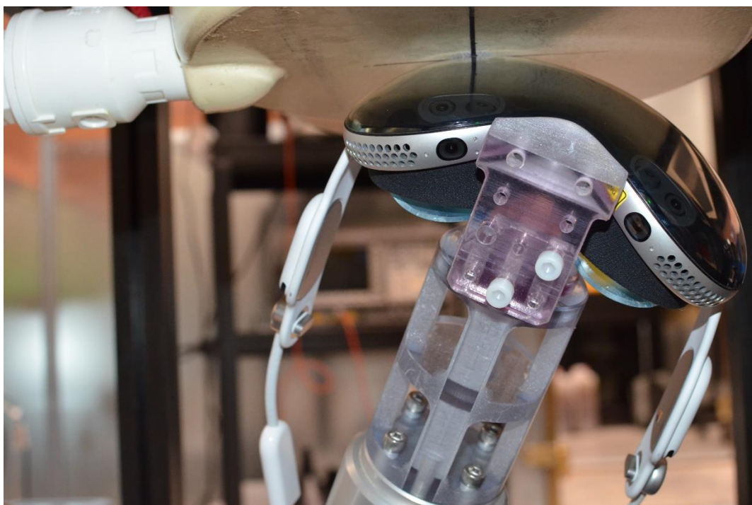
SAR Test Setup Photo 18: Antenna 1 Point 34 Extremity SAR at 0.0 cm
