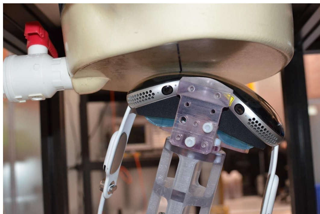
SAR Test Setup Photo 20: Antenna 1 Point 39 Extremity SAR at 0.0 cm
