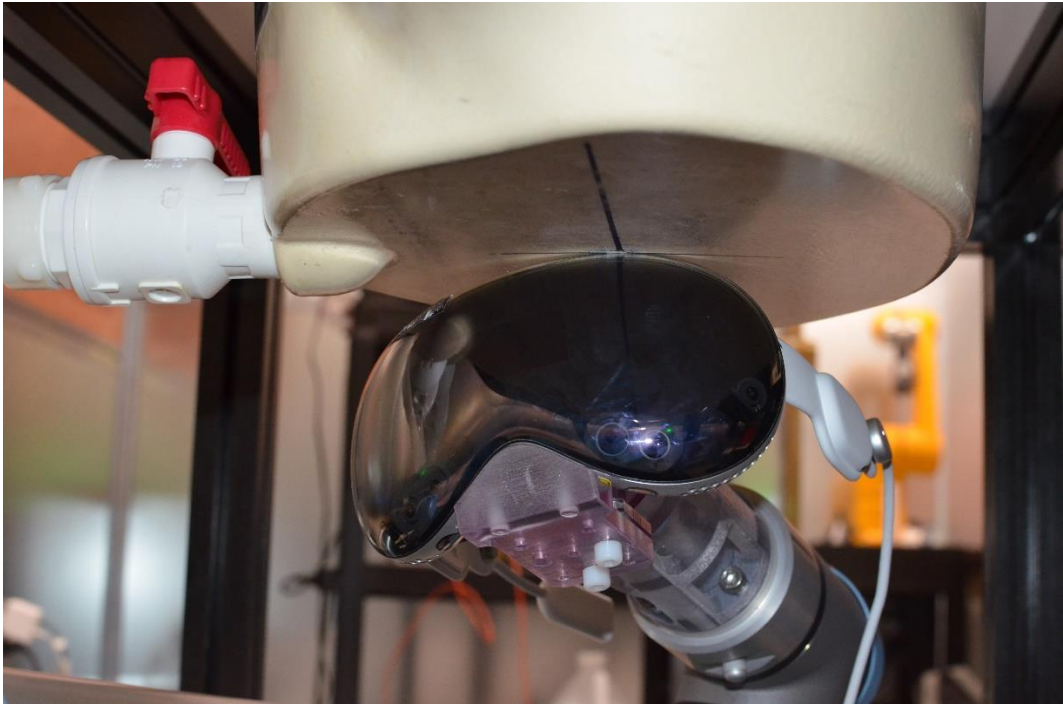
SAR Test Setup Photo 23: Antenna 2 Point 3 Extremity SAR at 0.0 cm
