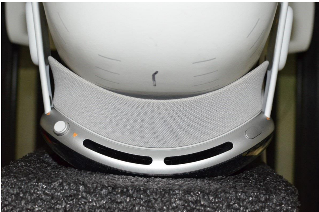
SAR Test Setup Photo 5: Antenna Testing with Mini Light Seal Head SAR at 0.0 cm
