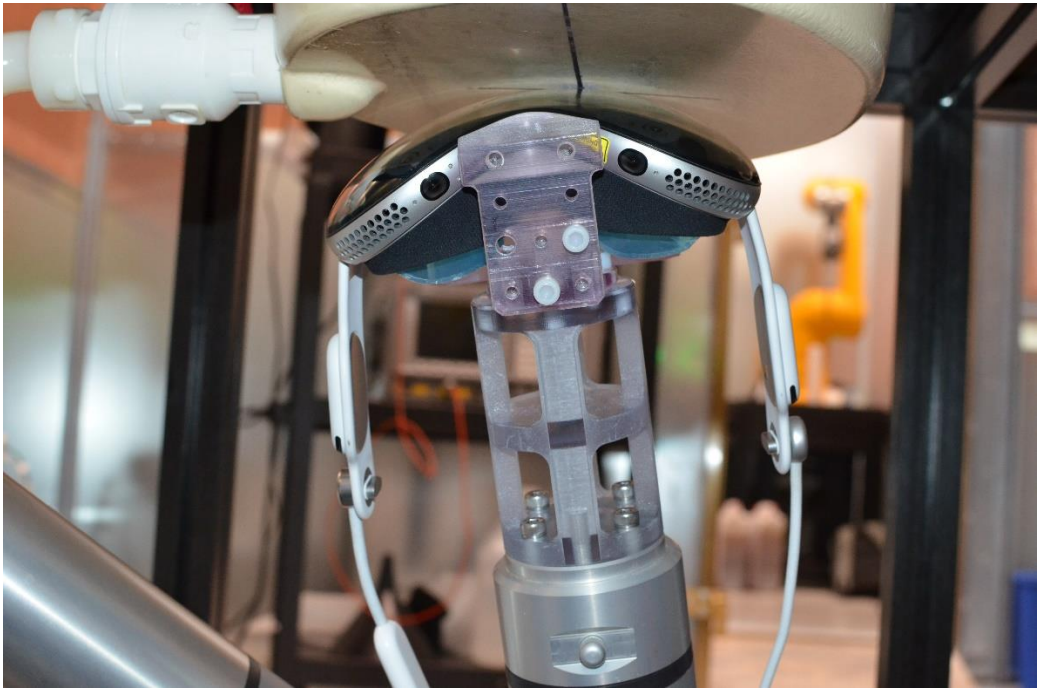
SAR Test Setup Photo 24: Antenna 2 Point 4 Extremity SAR at 0.0 cm
