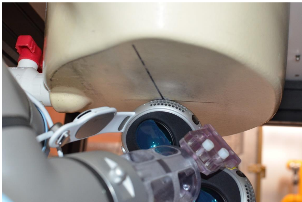
SAR Test Setup Photo 35: Antenna NB UNII_R Point 22 Extremity SAR at 0.0 cm
