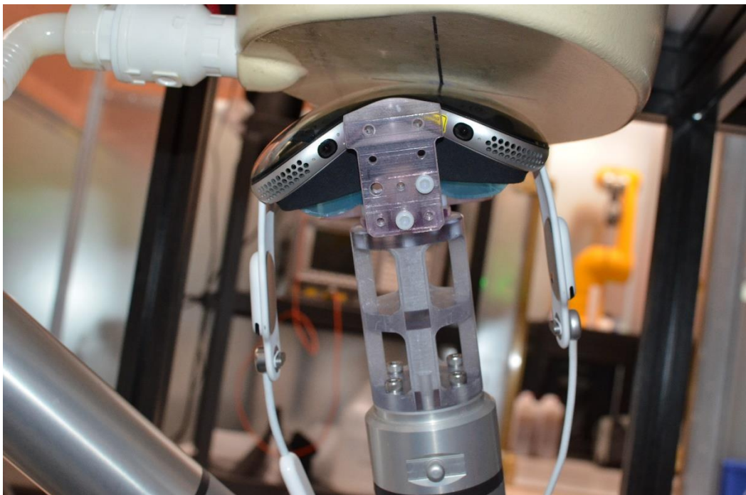
SAR Test Setup Photo 25: Antenna 2 Point 5 Extremity SAR at 0.0 cm
