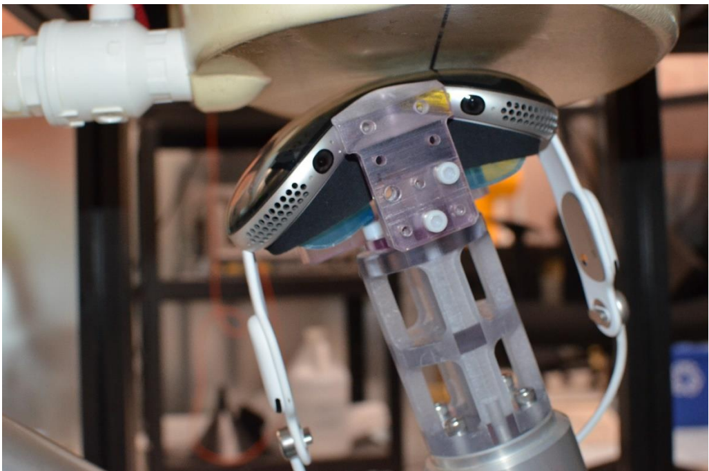
SAR Test Setup Photo 31: Antenna 2 Point 17 Extremity SAR at 0.0 cm
