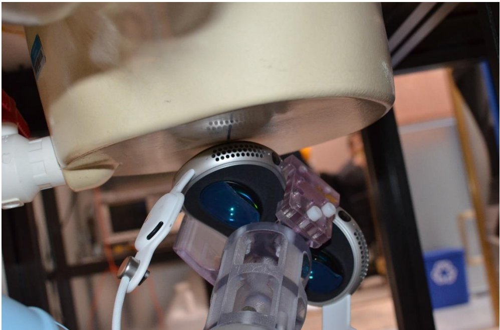
SAR Test Setup Photo 38: Antenna NB UNII_R Point 26 Extremity SAR at 0.0 cm
