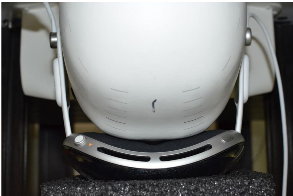
SAR Test Setup Photo 1: Antenna 1 and Antenna 2 Head SAR at 0.0 cm
