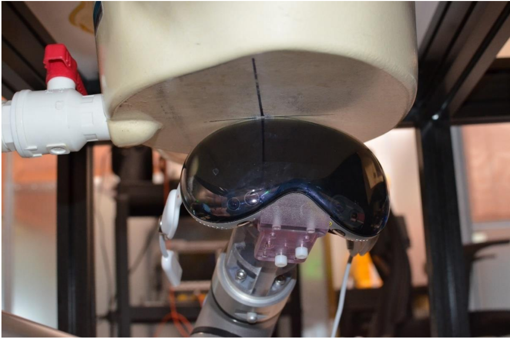
SAR Test Setup Photo 7: Antenna 1 Point 9 Extremity SAR at 0.0 cm
