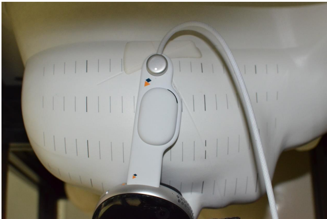
SAR Test Setup Photo 3: Antenna NB UNII_L Head SAR at 0.0 cm
