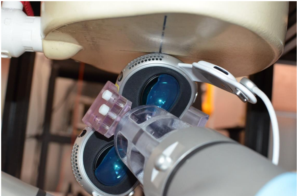
SAR Test Setup Photo 43: Antenna NB UNII_L Point 13 Extremity SAR at 0.0 cm
