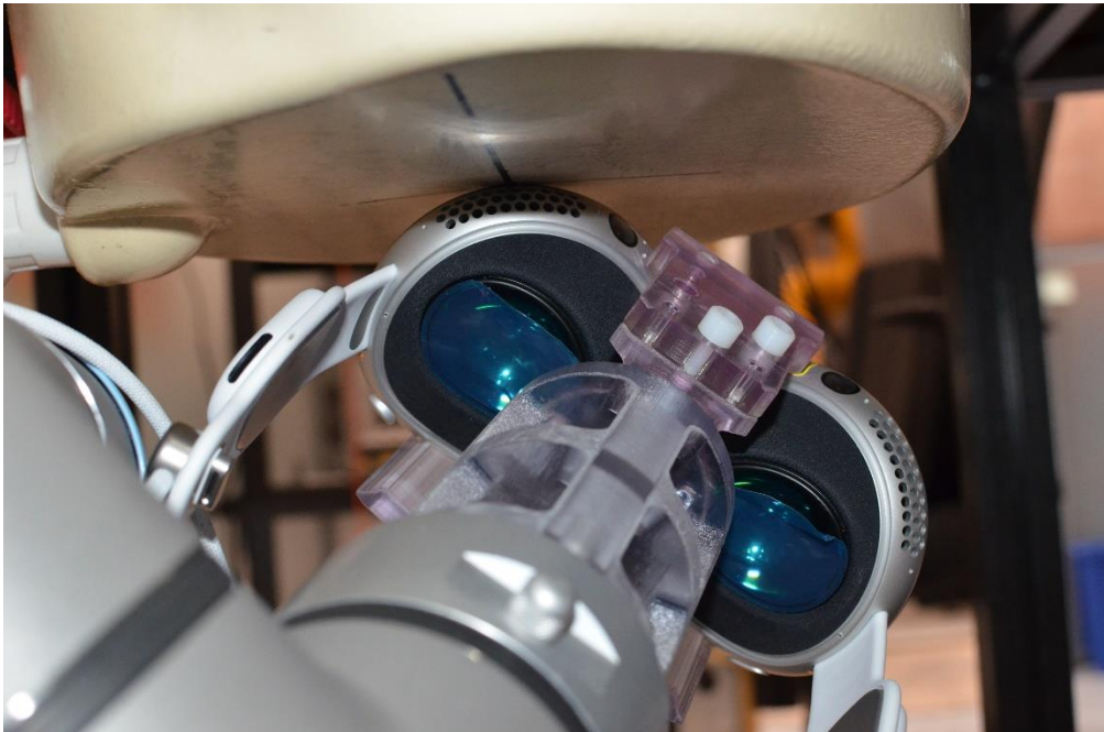
SAR Test Setup Photo 34: Antenna NB UNII_R Point 19 Extremity SAR at 0.0 cm
