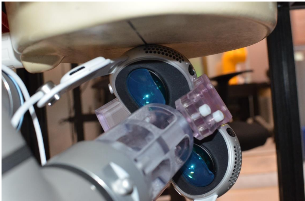
SAR Test Setup Photo 39: Antenna NB UNII_L Point 28 Extremity SAR at 0.0 cm
