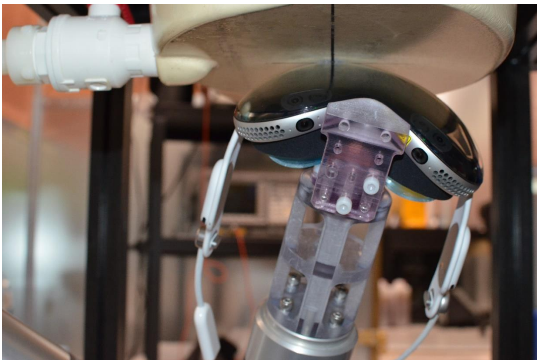
SAR Test Setup Photo 16: Antenna 1 Point 32 Extremity SAR at 0.0 cm
