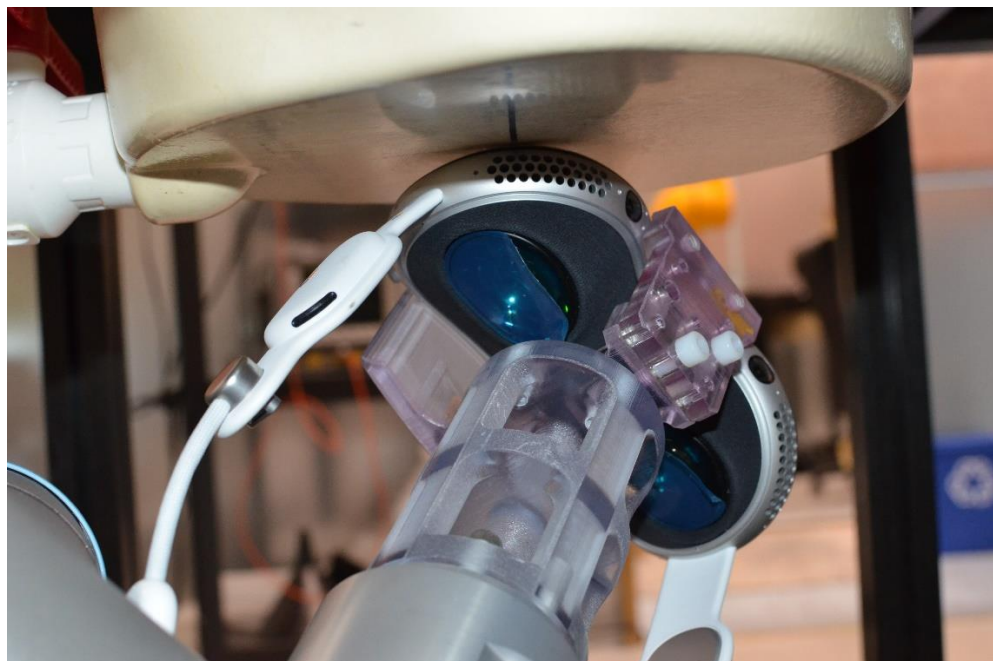
SAR Test Setup Photo 36: Antenna NB UNII_R Point 23 Extremity SAR at 0.0 cm
