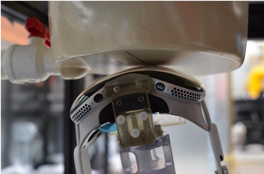
SAR Test Setup Photo 44: Antenna Testing with Main Light Seal Extremity SAR at 0.0 cm
