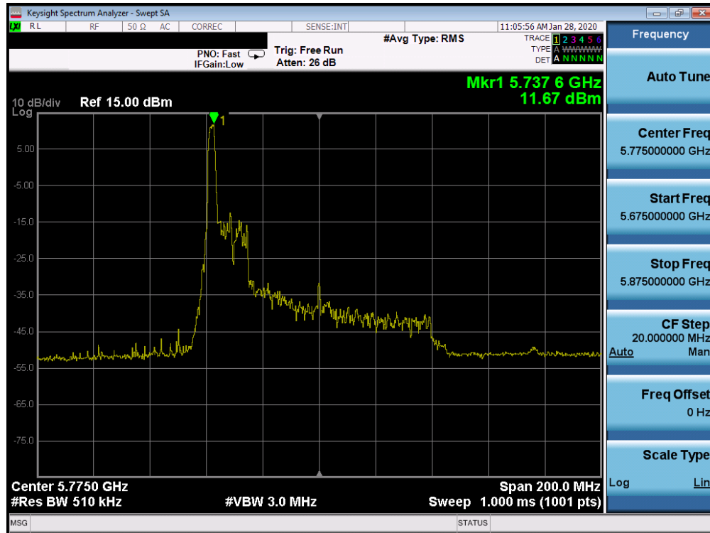
Plot 7-333. Power Spectral Density Plot SISO CORE 0 (80MHz BW 802.11ax Index 0 – RU26 (UNII Band 3) – Ch. 155)
