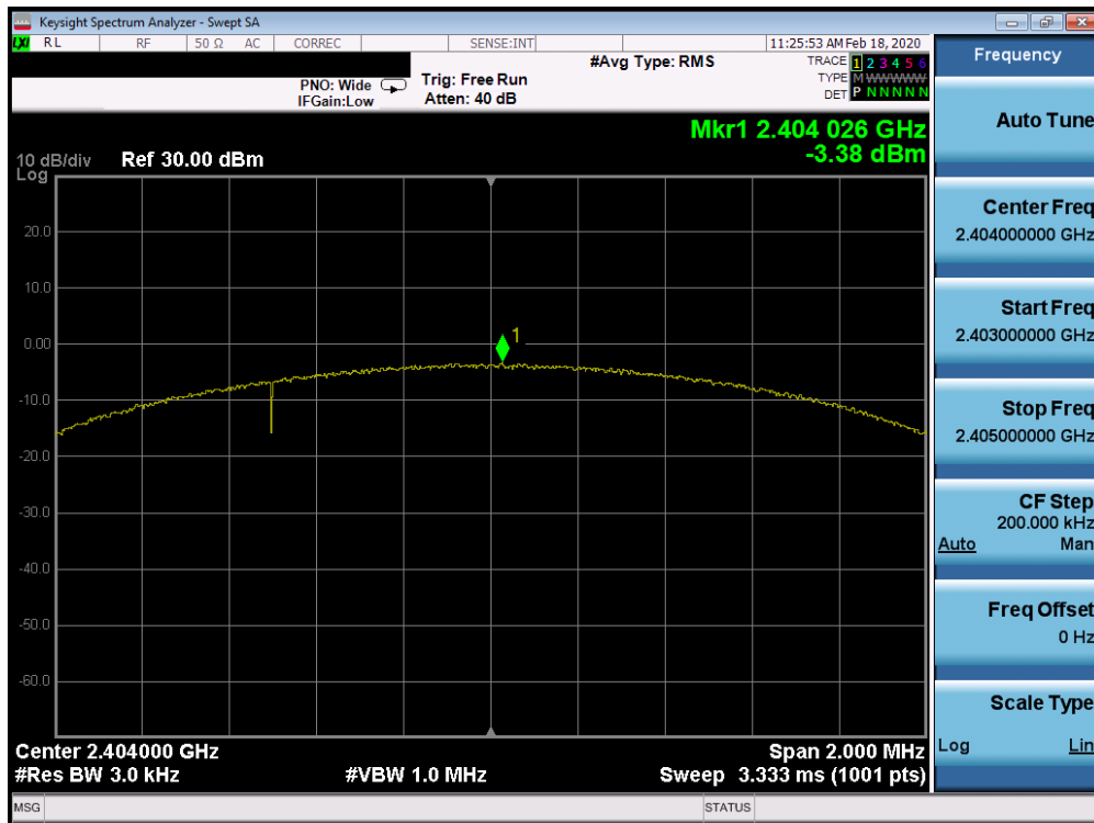
Plot 7-50. Power Spectral Density Plot Tx BF Ant 2a (Bluetooth (LE), 2Mbps, ePA – Ch. 1)
