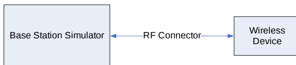
Figure 8-2 Power Measurement Setup
