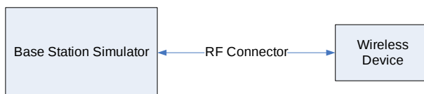
Figure 8-1 Power Measurement Setup
