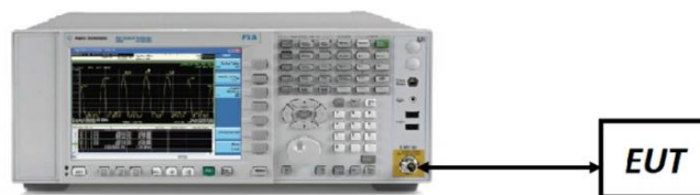
Figure 7-4. Test Instrument & Measurement Setup
