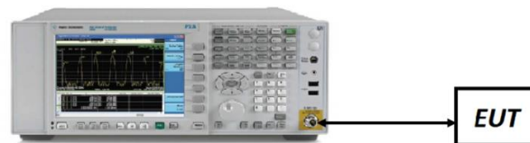
Figure 7-1. Test Instrument & Measurement Setup
