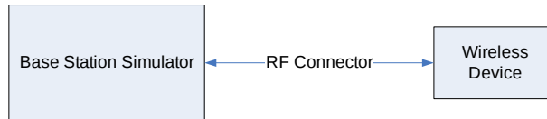
Figure 8-2 Power Measurement Setup
