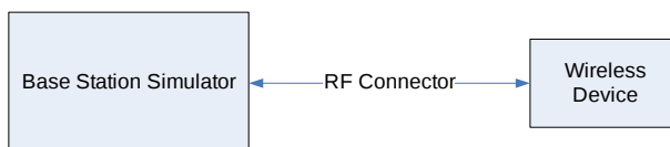
Figure 8-1 Power Measurement Setup
