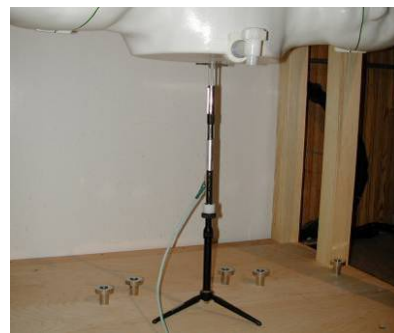
Figure 9-2 System Verification Setup Photo
