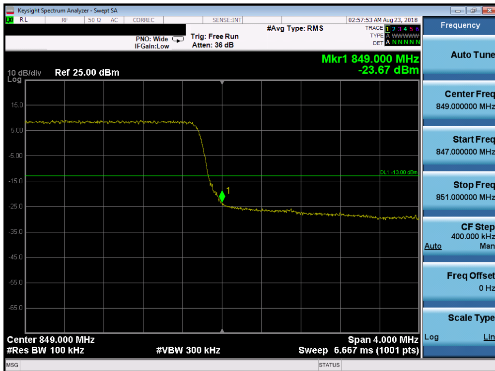
Plot 7-217. Upper Band Edge Plot (Band 5 – 5.0MHz QPSK – RB Size 25)
