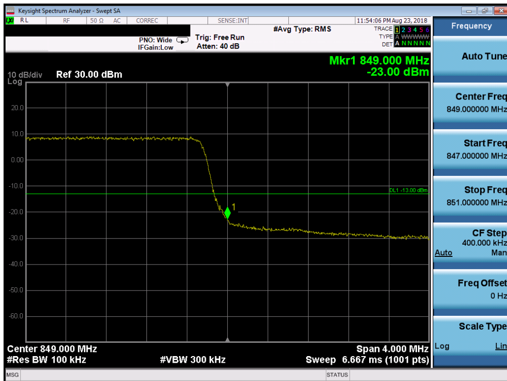
Plot 7-225. Upper Band Edge Plot (Band 5 - 5.0MHz QPSK - RB Size 25)
