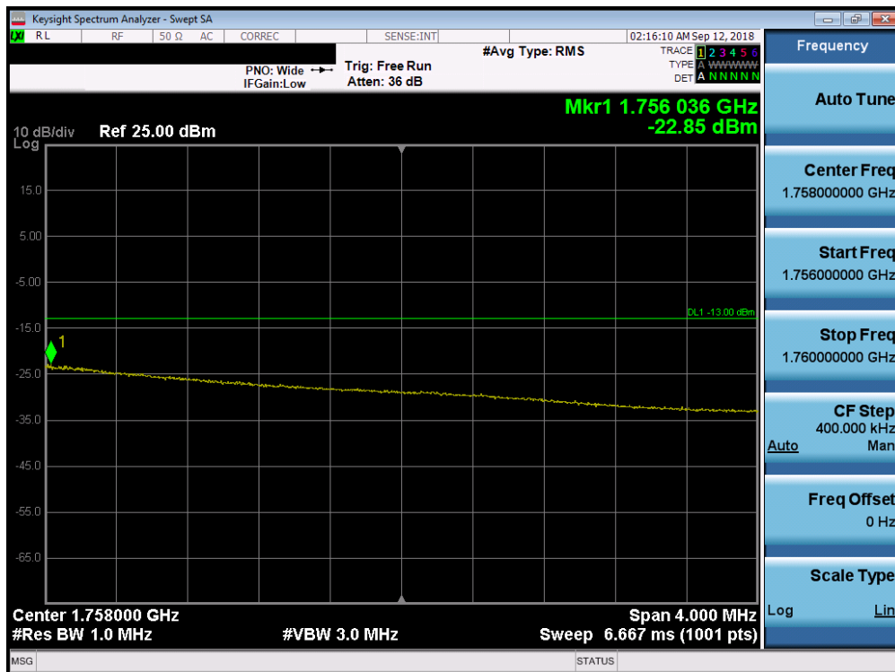
Plot 7-249. Upper Extended Band Edge Plot (Band 4 – 15.0MHz QPSK – RB Size 75)
