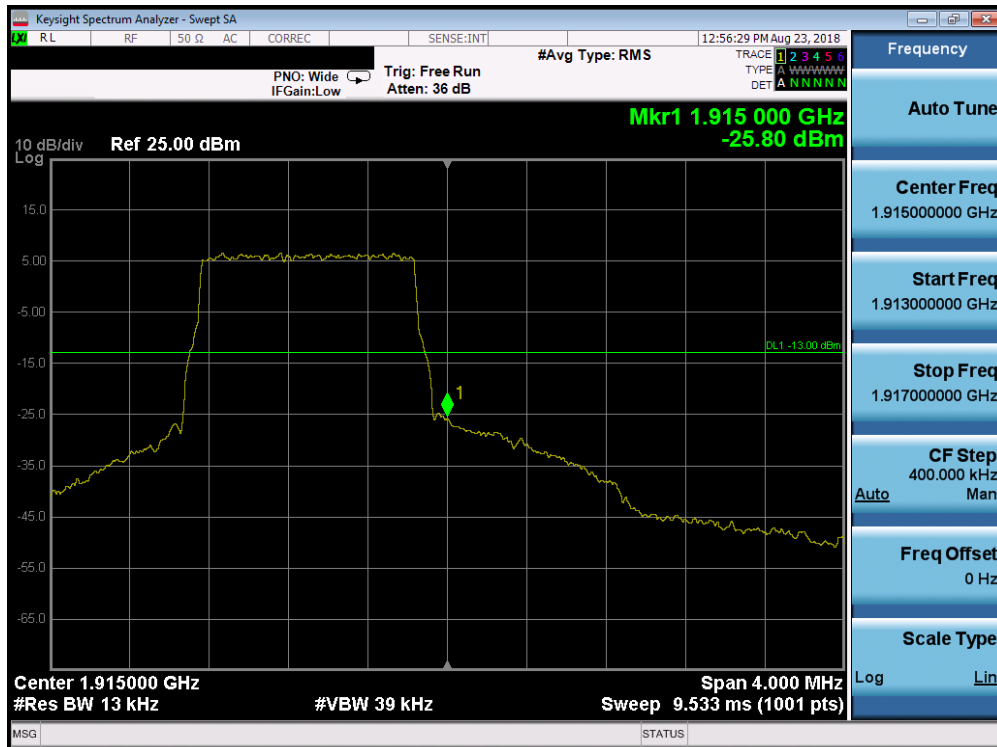
Plot 7-304. Upper Band Edge Plot (Band 25 – 1.4MHz QPSK – RB Size 6)
