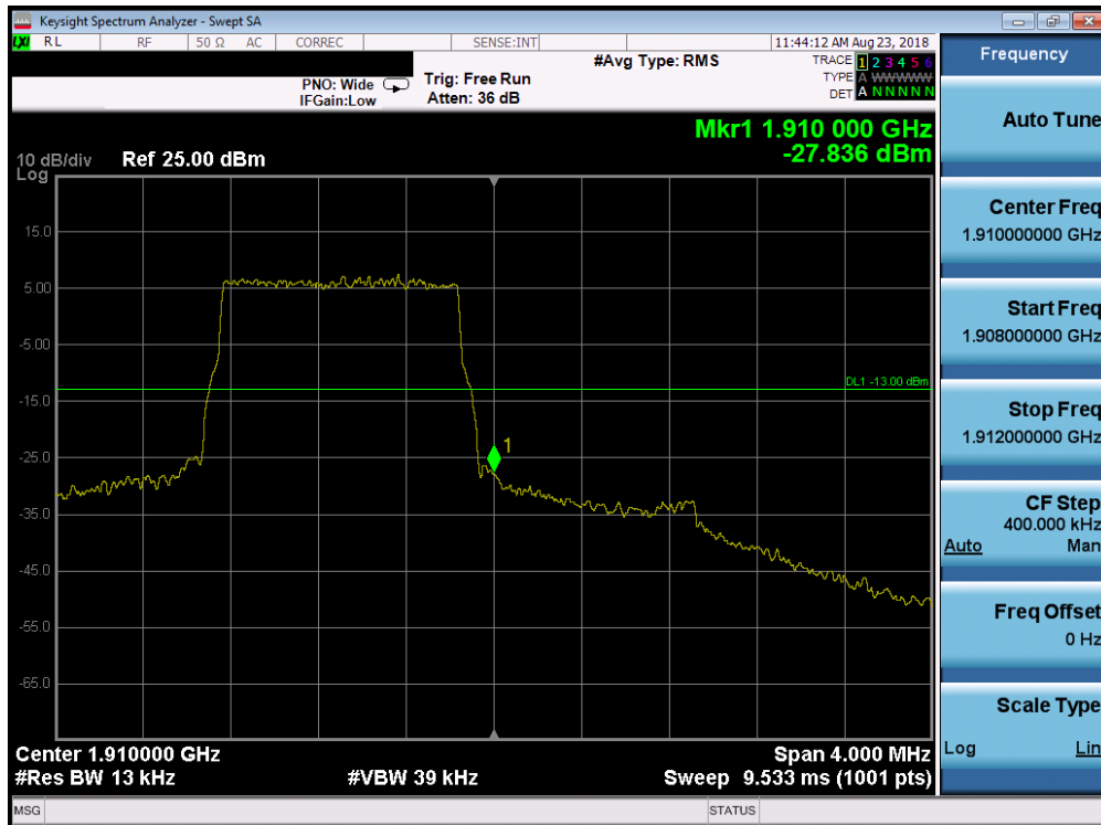
Plot 7-280. Upper Band Edge Plot (Band 2 – 1.4MHz QPSK – RB Size 6)
