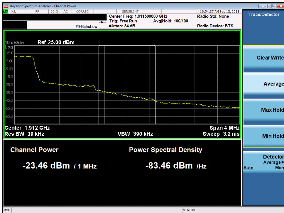
Plot 7-281. Upper Extended Band Edge Plot (Band 2 – 1.4MHz QPSK – RB Size 6)
