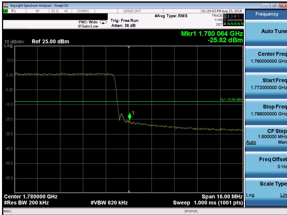
Plot 7-276. Upper Band Edge Plot (Band 66 – 20.0MHz QPSK – RB Size 100)
