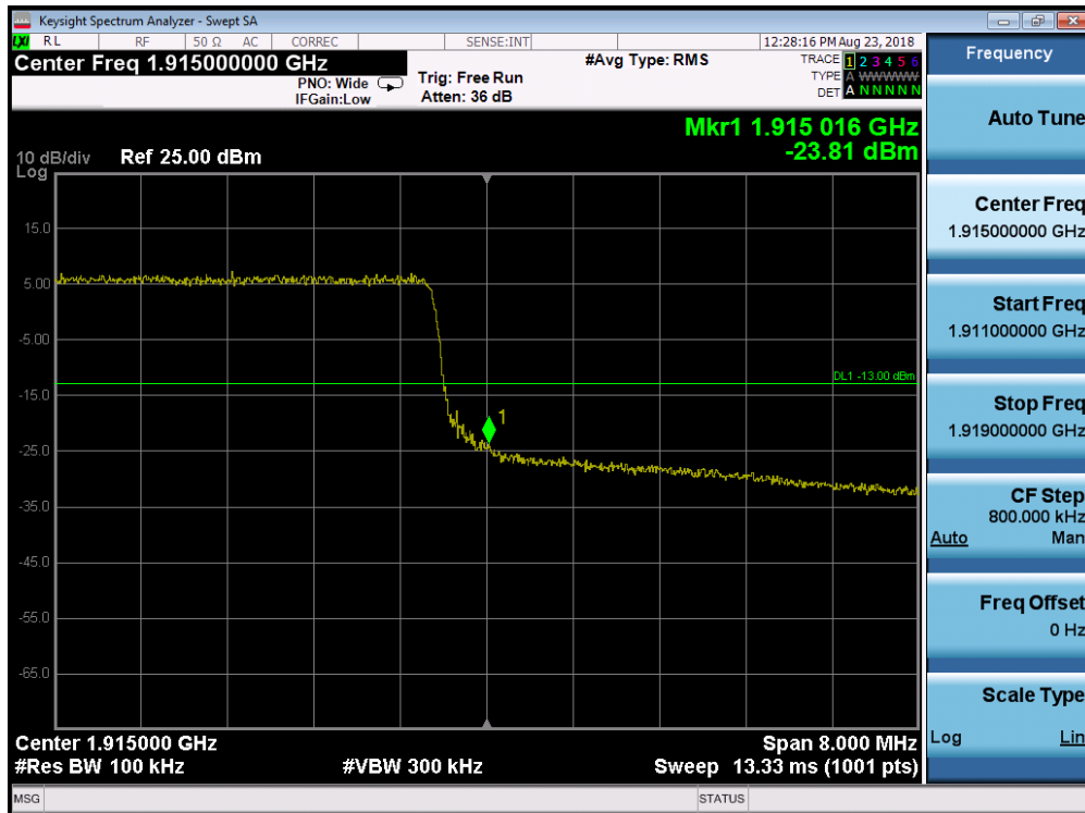
Plot 7-316. Upper Band Edge Plot (Band 25 – 10.0MHz QPSK – RB Size 50)
