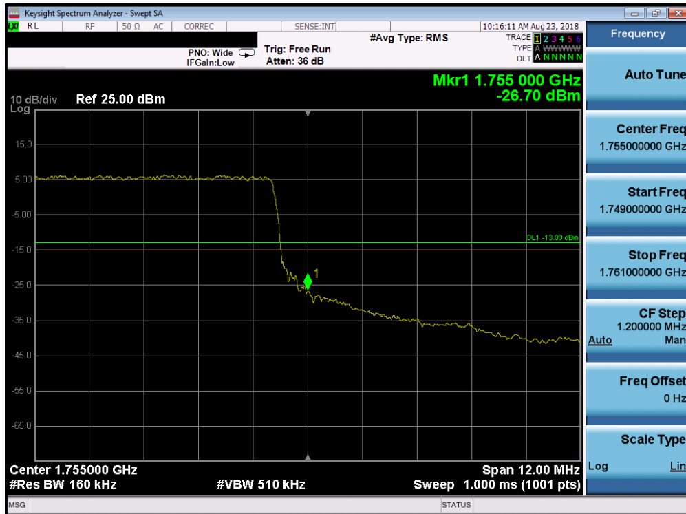
Plot 7-248. Upper Band Edge Plot (Band 4 – 15.0MHz QPSK – RB Size 75)
