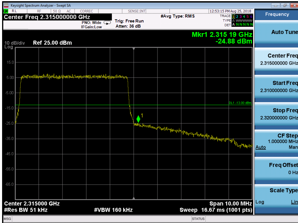
Plot 7-328. Upper Band Edge Plot (Band 30 – 5.0MHz QPSK – RB Size 25)
