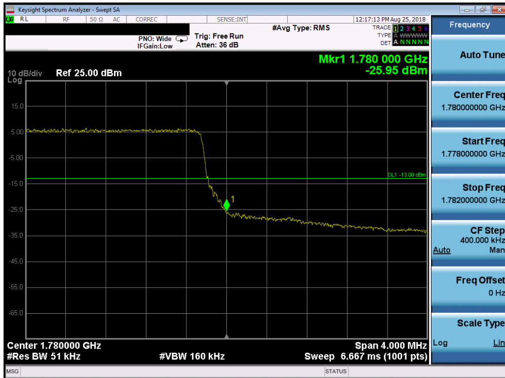
Plot 7-264. Upper Band Edge Plot (Band 66 – 5.0MHz QPSK – RB Size 25)
