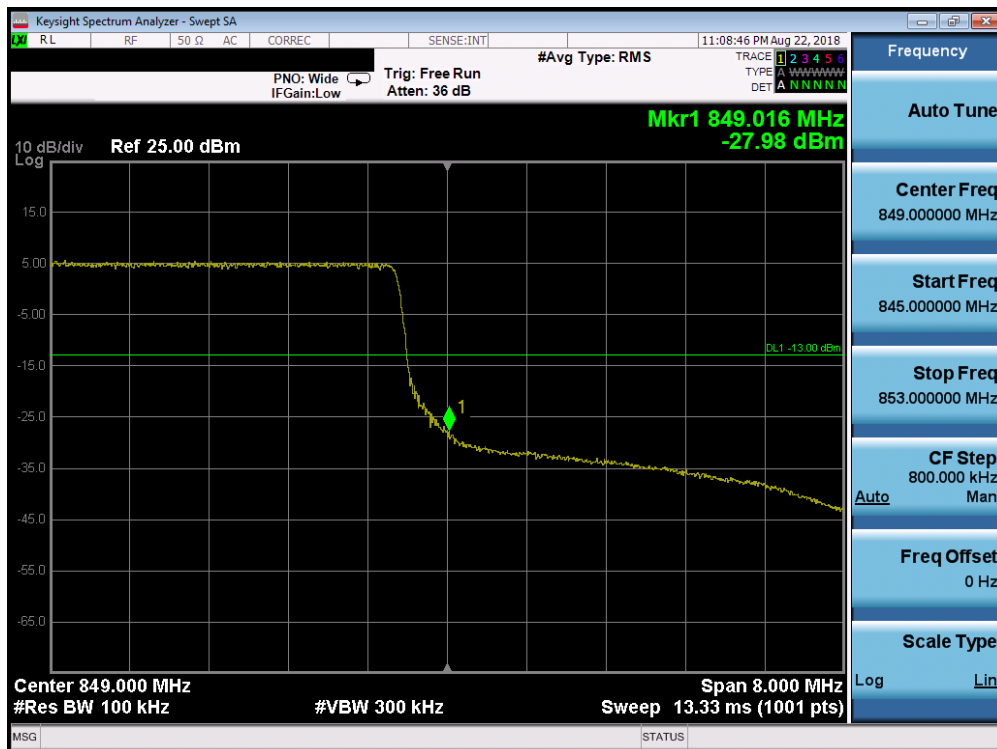
Plot 7-219. Upper Band Edge Plot (Band 5 – 10.0MHz QPSK – RB Size 50)
