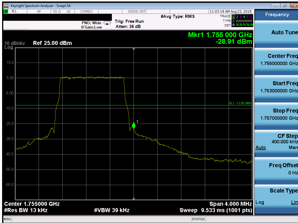
Plot 7-232. Upper Band Edge Plot (Band 4 – 1.4MHz QPSK – RB Size 6)
