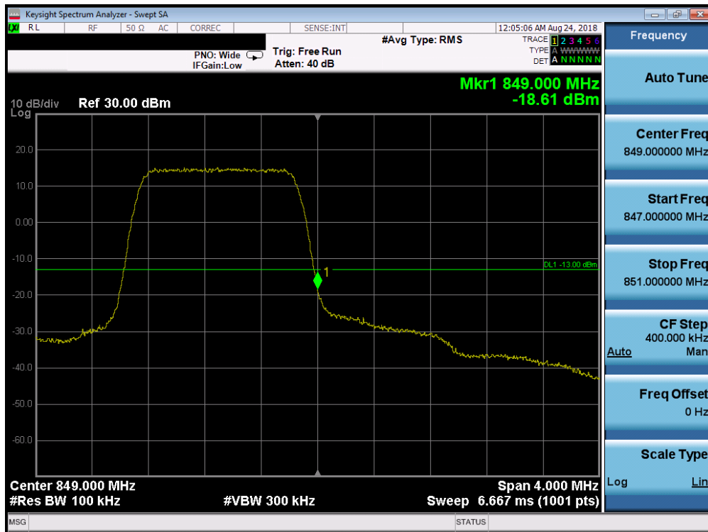
Plot 7-221. Upper Band Edge Plot (Band 5 – 1.4MHz QPSK – RB Size 6)
