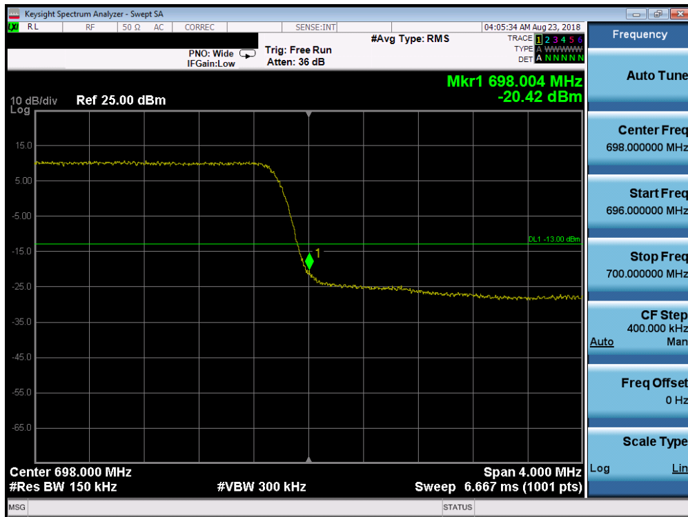
Plot 7-185. Upper Band Edge Plot (Band 71 – 5.0MHz QPSK – RB Size 25)
