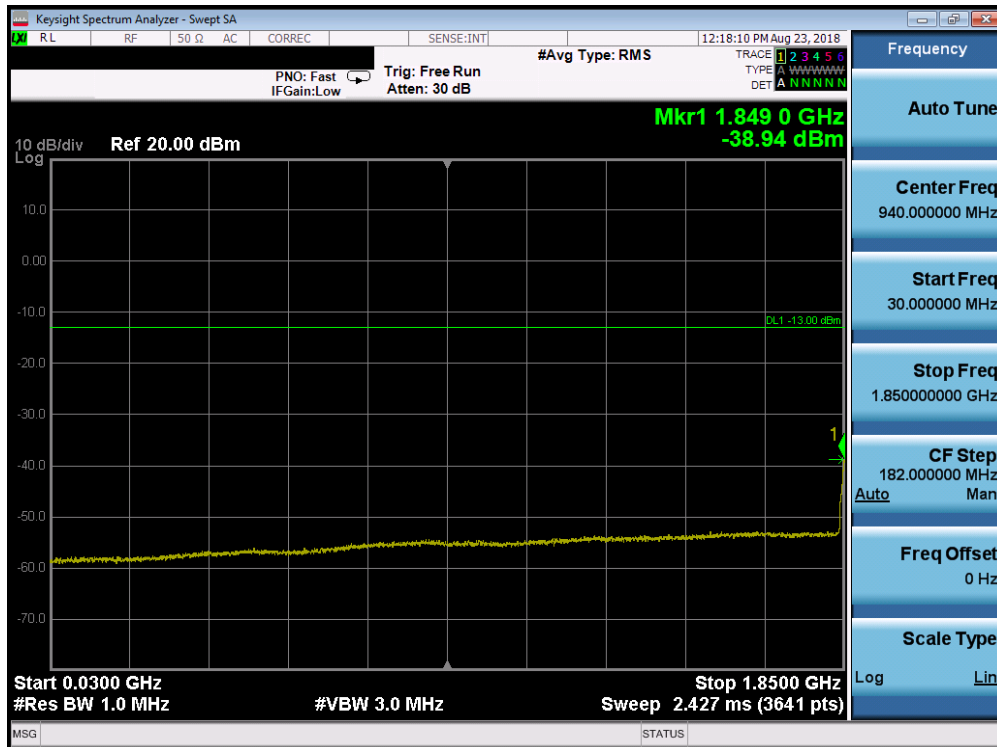
Plot 7-160. Conducted Spurious Plot (Band 25/2 – 20.0MHz QPSK – RB Size 1, RB Offset 0 – High Channel)
