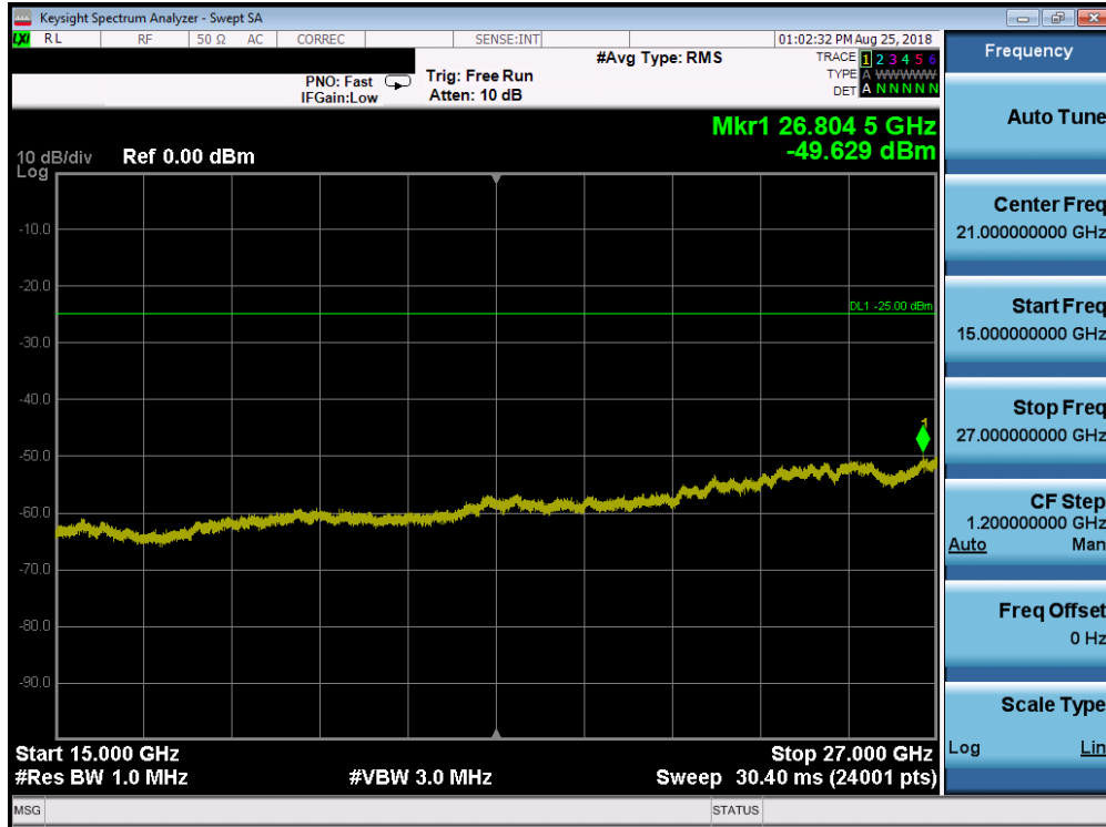
Plot 7-174. Conducted Spurious Plot (Band 7 – 20.0MHz QPSK – RB Size 1, RB Offset 0 – High Channel)
