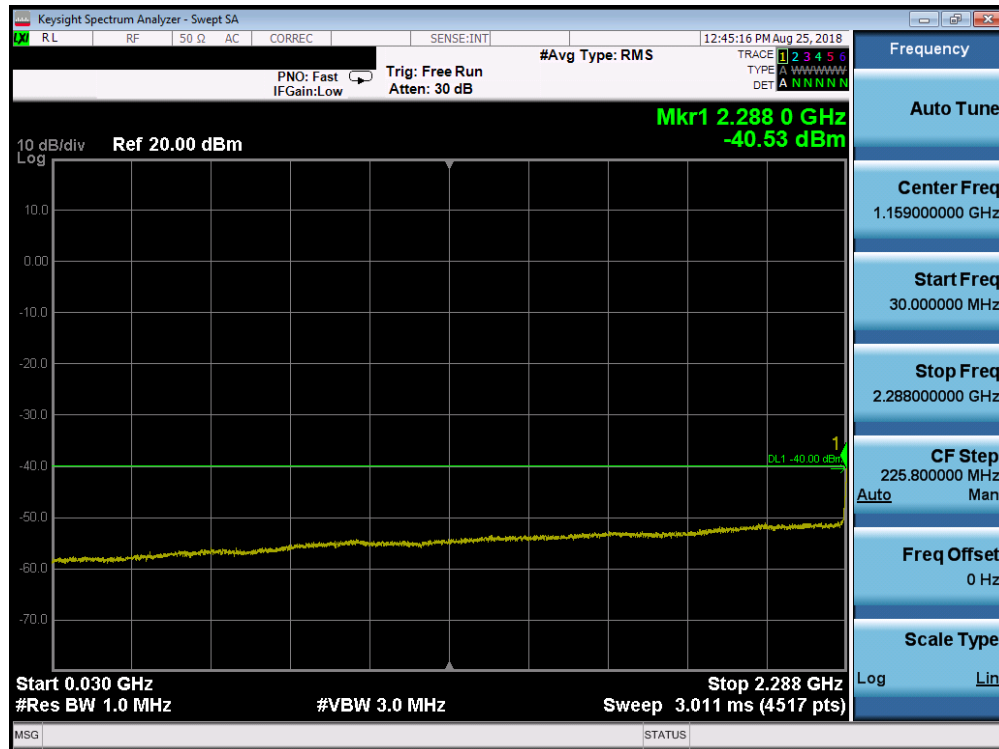
Plot 7-163. Conducted Spurious Plot (Band 30 – 10.0MHz QPSK – RB Size 1, RB Offset 0 – Mid Channel)
