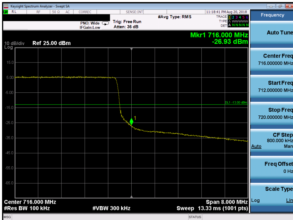
Plot 7-199. Upper Band Edge Plot (Band 12 – 10.0MHz QPSK – RB Size 50)
