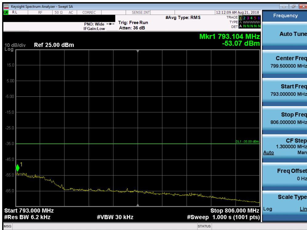
Plot 7-207. Upper Emission Mask Edge Plot (Band 13 – 5.0MHz QPSK – RB Size 25)
