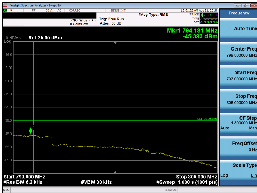
Plot 7-211. Upper Emission Mask Edge Plot (Band 13 – 10.0MHz QPSK – RB Size 50)
