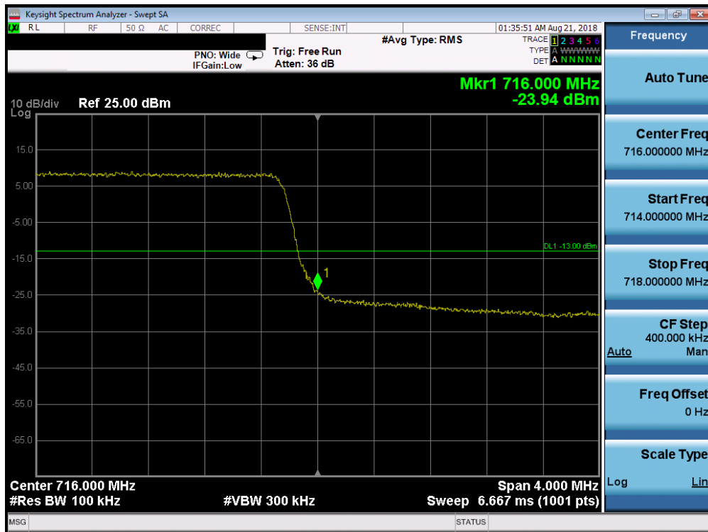
Plot 7-201. Upper Band Edge Plot (Band 17 – 5.0MHz QPSK – RB Size 25)
