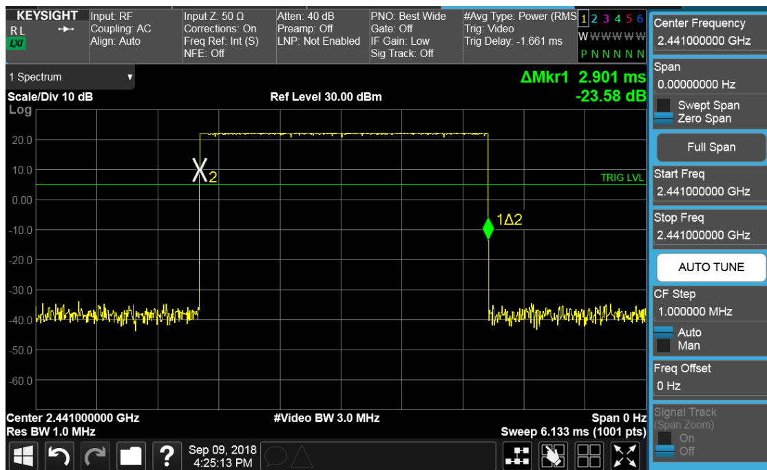
Plot 7-52. Time of Occupancy Plot ANT1(Bluetooth, 8DPSK, ePA)
