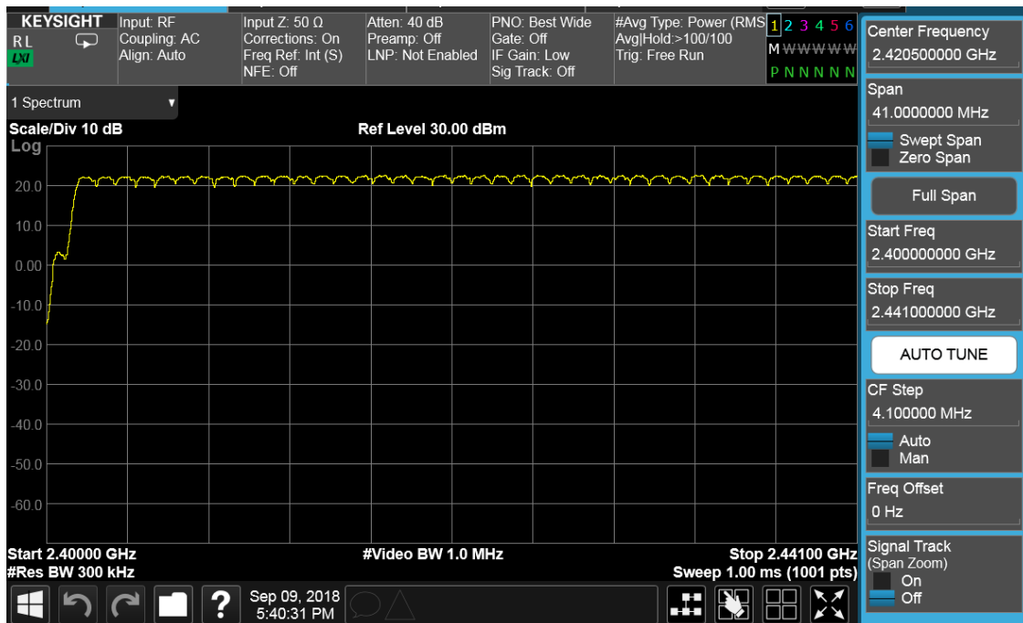
Plot 7-65. Low End Spectrum Channel Hopping Plot ANT2 (Bluetooth, 8DPSK, ePA)
