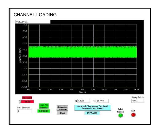
The level of traffic loading on the channel by the EUT is 19.776%
