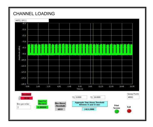
The level of traffic loading on the channel by the EUT is 24.132%
