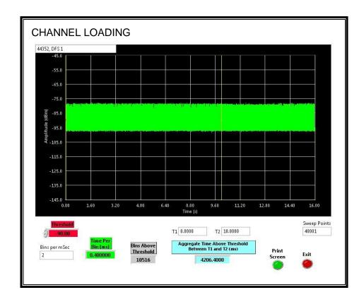
The level of traffic loading on the channel by the EUT is 42.064%
