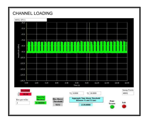
The level of traffic loading on the channel by the EUT is 22.28%%
