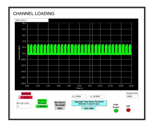
The level of traffic loading on the channel by the EUT is 19.612%
