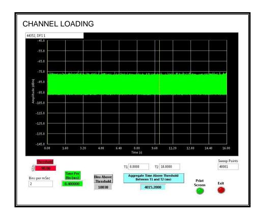
The level of traffic loading on the channel by the EUT is 40.152%
