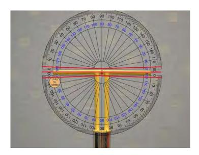
$\bullet$  The center red line indicates that the arms of the dipole fall within  $\pm 2^\circ$
