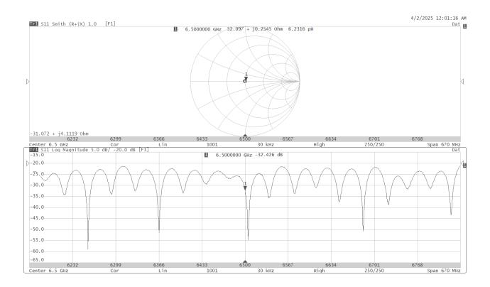
• Return/Loss is greater than the -20 dB cutoff and Impedance is within 5  $\Omega$  of previous value.
