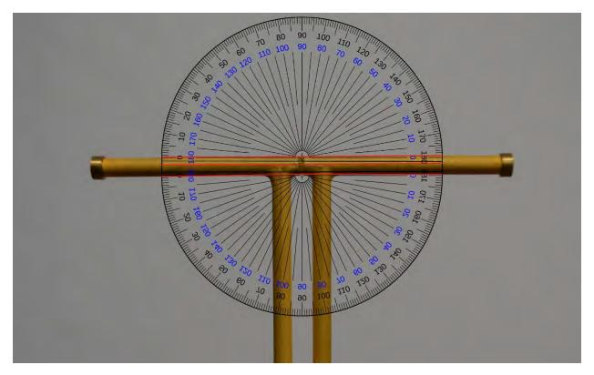
• The center red line indicates that the arms of the dipole fall within  $\pm 2^\circ$
