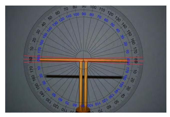
• The center red line indicates that the arms of the dipole fall within  $\pm 2^{\circ}$
