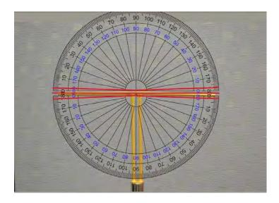
$\bullet~$  The center red line indicates that the arms of the dipole fall within  $\pm 2^{\circ}$
