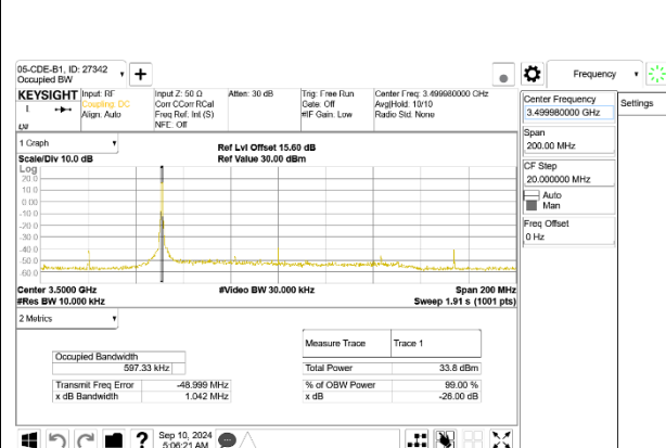
5G NR n77 100MHz BPSK Middle Channel RB1-0
