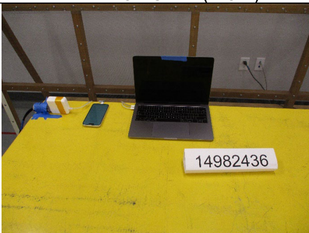
AC LINE CONDUCTED WITH HOST (FRONT)
