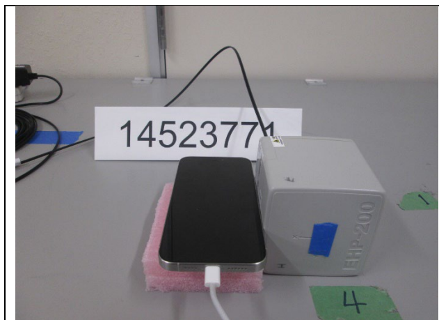
S1, RF Exposure Setup Photo
