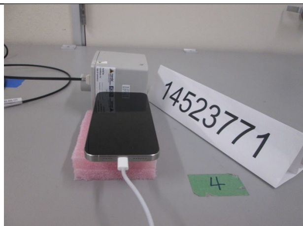
S2, RF Exposure Setup Photo
