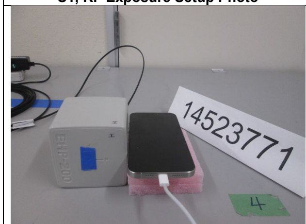
S3, RF Exposure Setup Photo
