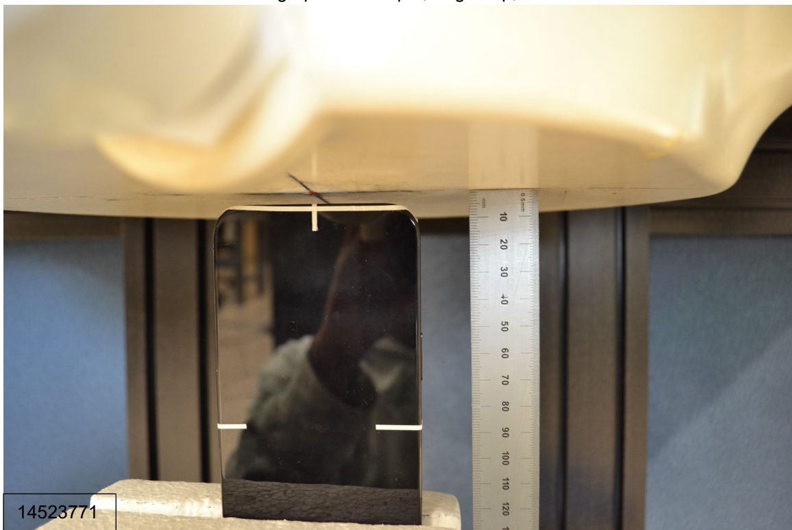
Photograph 12: Hotspot, Edge Top, 5 mm
