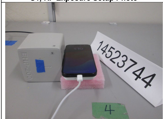
S3, RF Exposure Setup Photo
