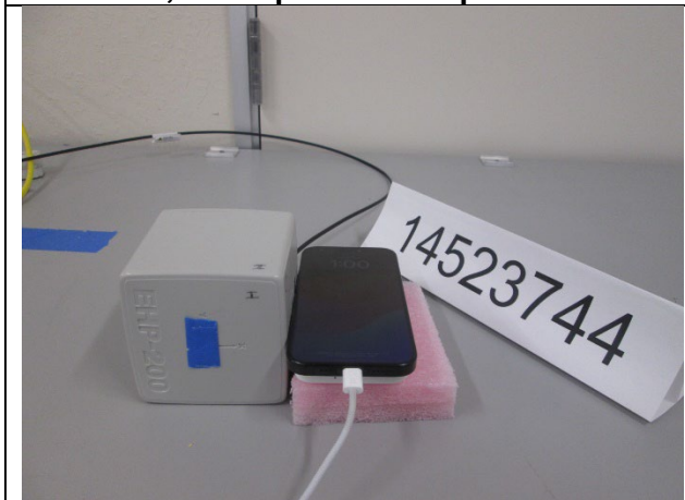
S3, RF Exposure Setup Photo
