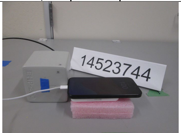
S4, RF Exposure Setup Photo
