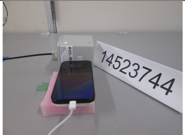
S2, RF Exposure Setup Photo
