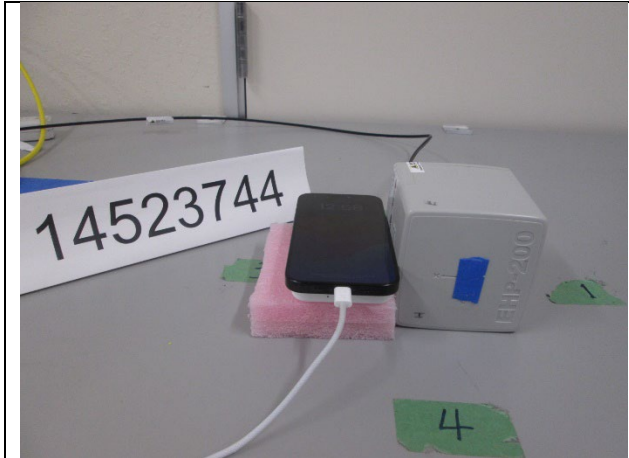
S1, RF Exposure Setup Photo
