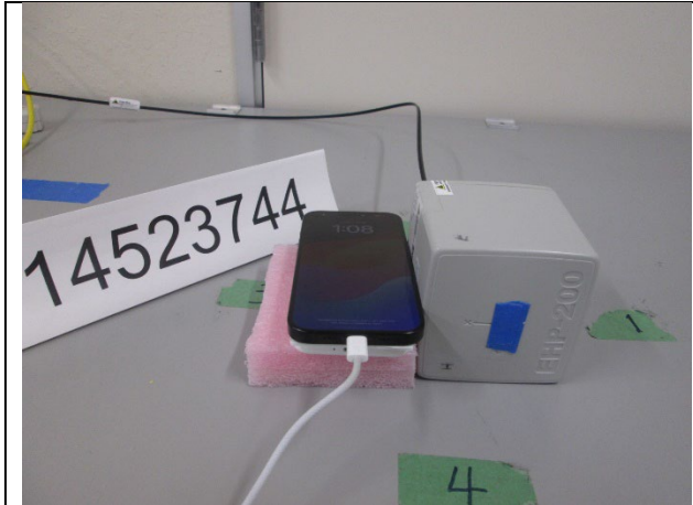
S1, RF Exposure Setup Photo
