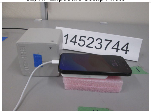
S4, RF Exposure Setup Photo
