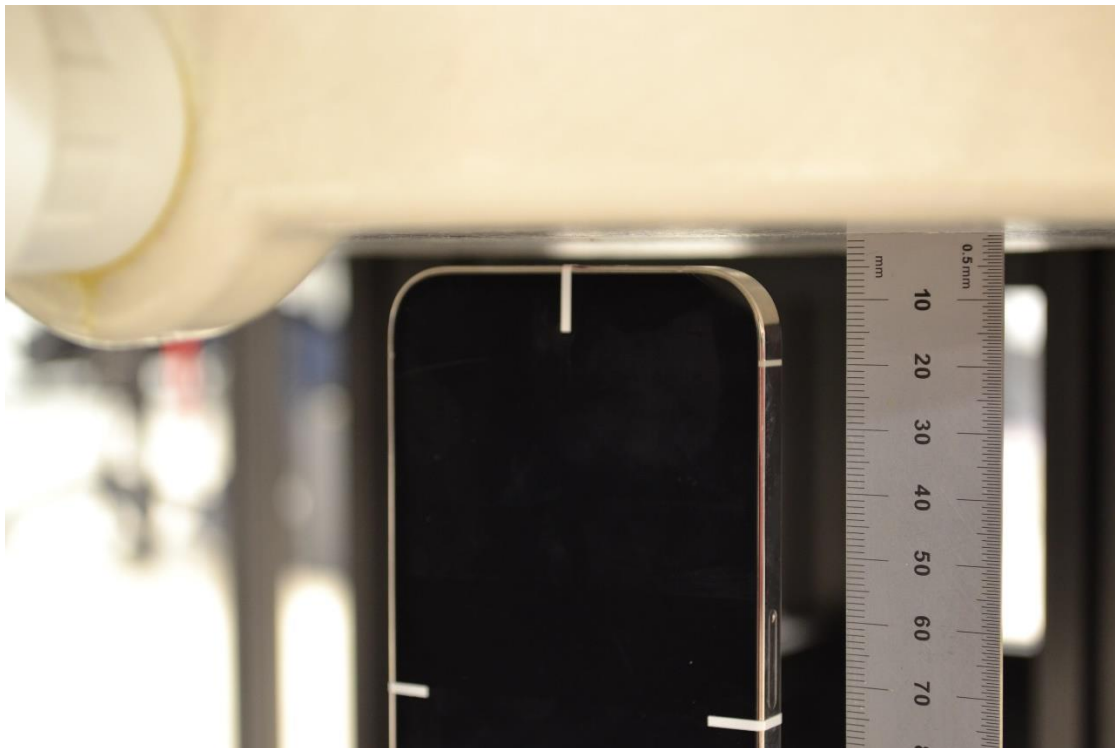
Figure 7-1: SAR measurement setup
