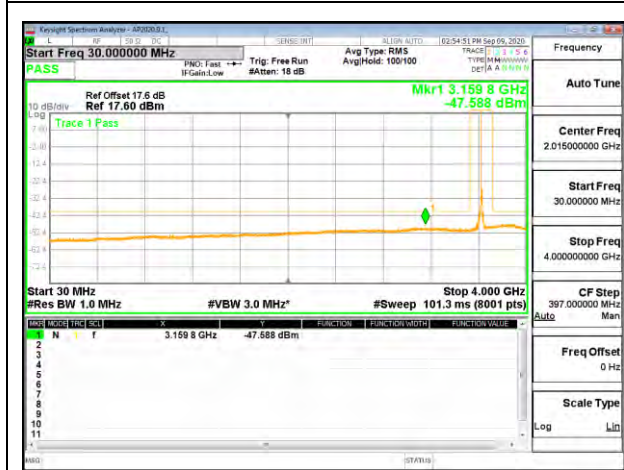
LTE B48 10MHz QPSK Mid Channel RB1-0 (30MHz to 4GHz)
