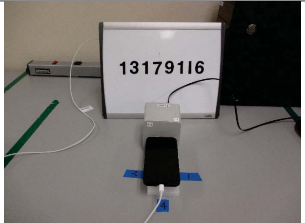
S2, RF Exposure Setup Photo
