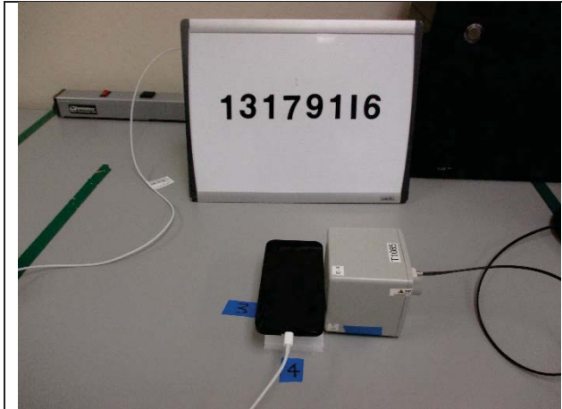
S1, RF Exposure Setup Photo
