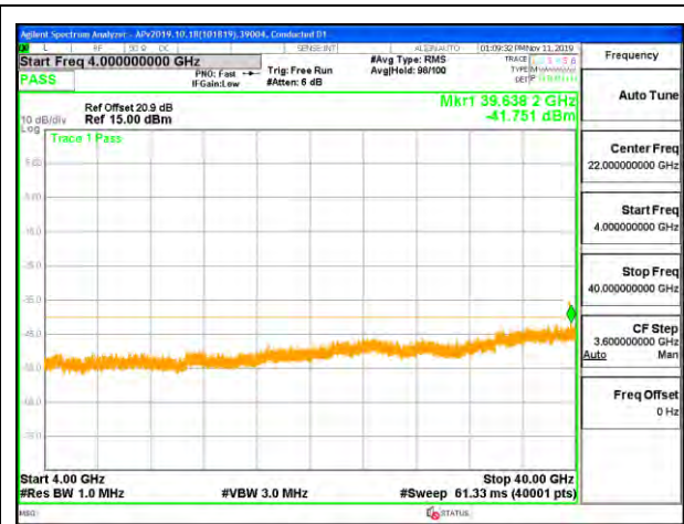
LTE B48 5MHz 16QAM Middle Channel RB1-0 (4G to 40G)
