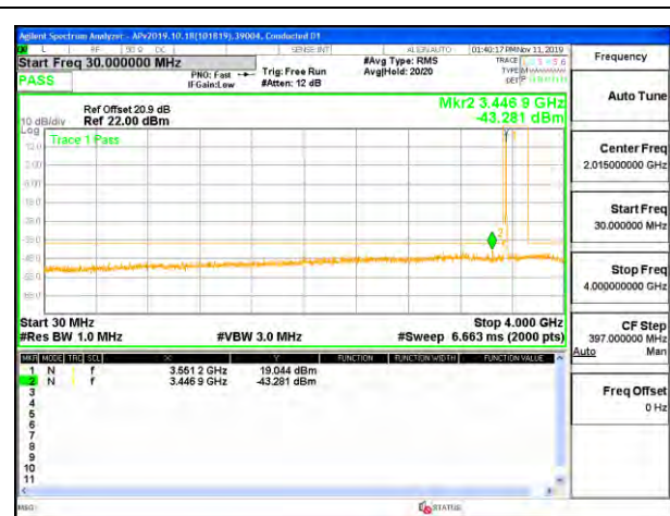
LTE B48 10MHz 16QAM Low Channel RB1-0 (30MHz to 4GHz)
