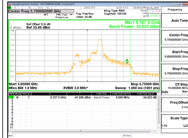
CHANNEL 142 ANT 4 POWER
