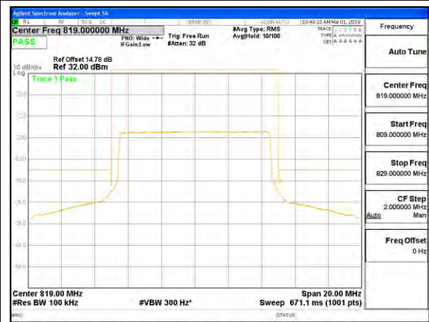
LTE B26 10MHz 16QAM Middle Channel RB50-0 ID:12491
