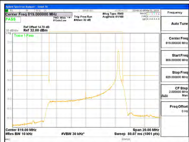
LTE B26 10MHz 16QAM Middle Channel RB1-49 ID:12491
