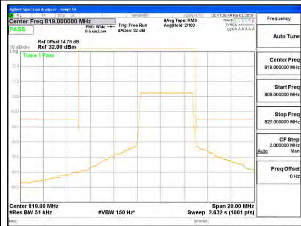
LTE B26 5MHz 16QAM High Channel RB25-0 ID:12491
