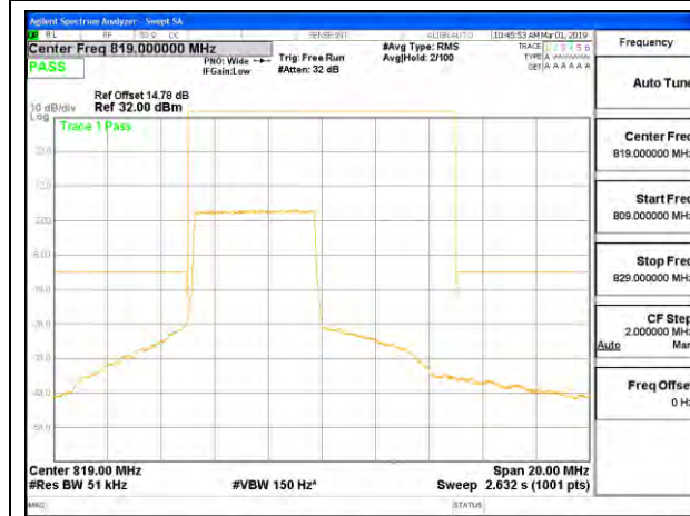
LTE B26 5MHz 16QAM Low Channel RB25-0 ID:12491
